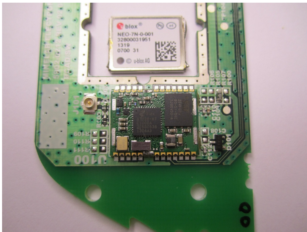
Figure 1a. GPS Receiver with can removed
