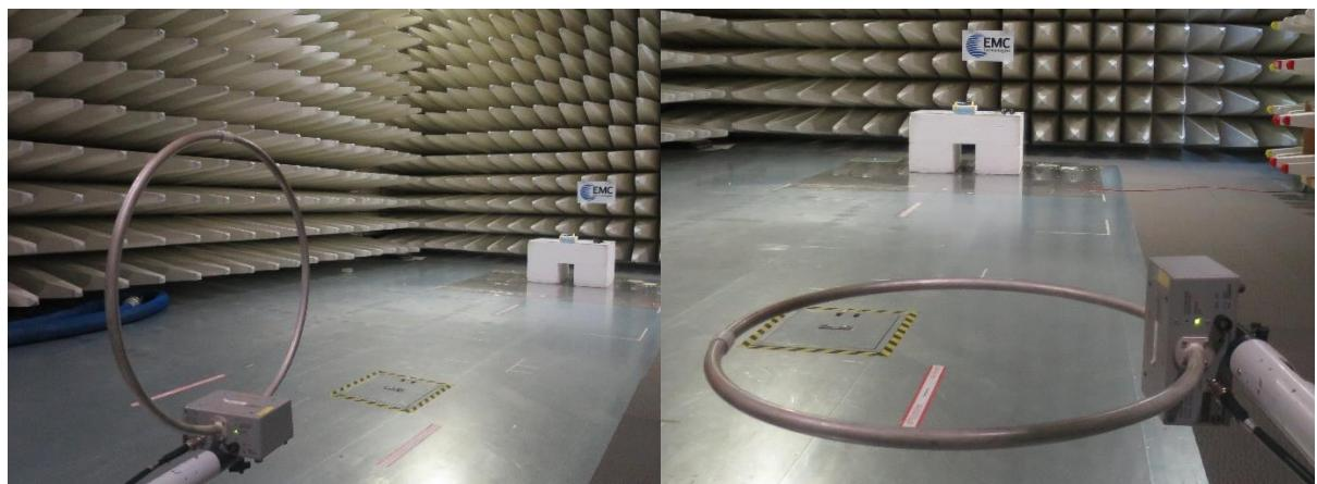
Radiated Emissions - 30 MHz to 1000 MHz
