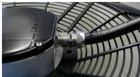
If the connection of the conduits is not possible with the thread adapter due to a lack of installation space, Ziehl-Abegg recommends its customers use an UL514B approved flexible connection hose system.
