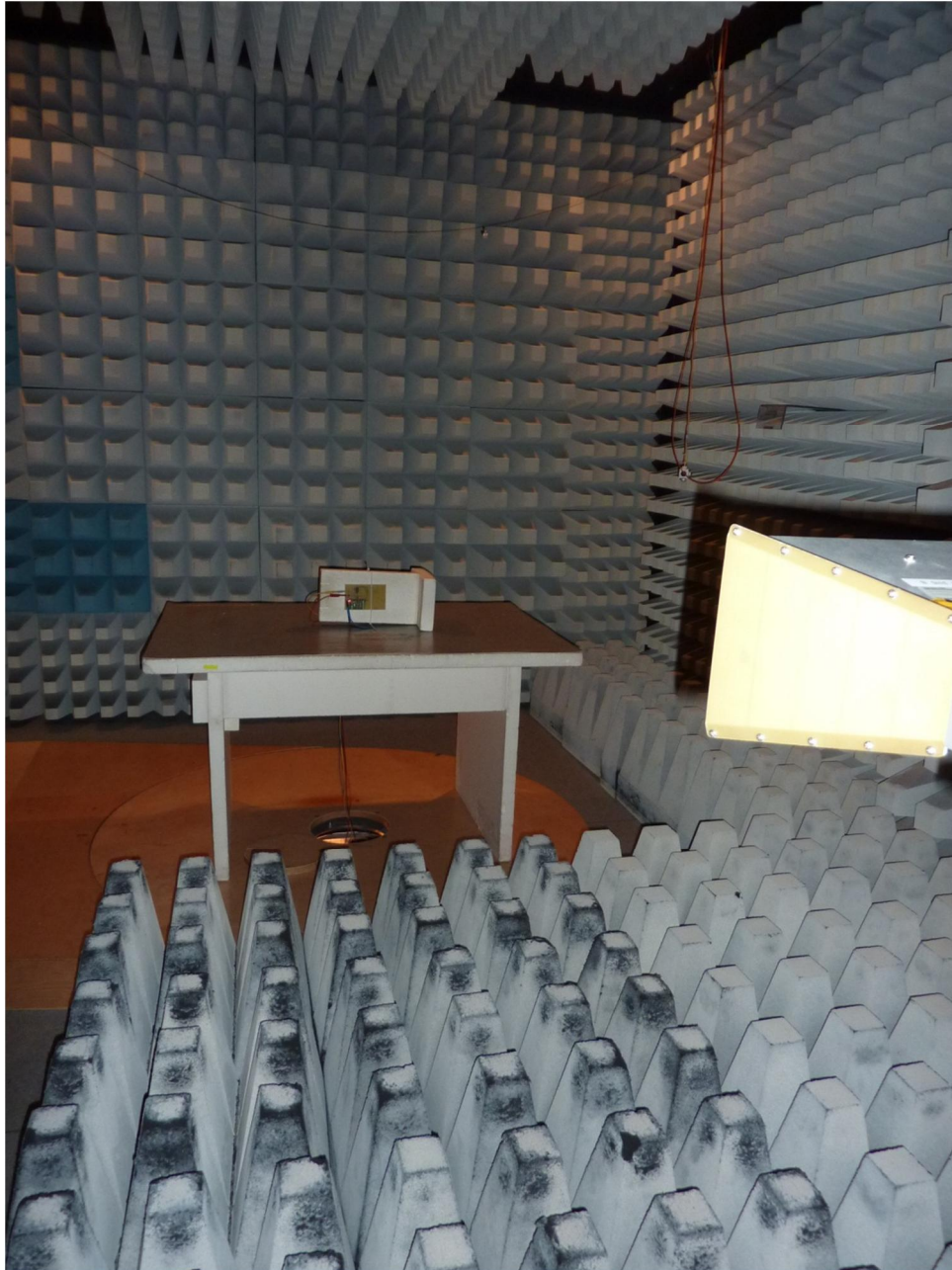
113482_9: Test setup fully anechoic chamber
