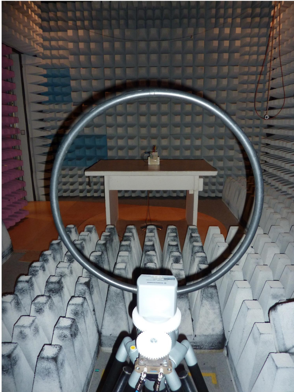
113482_7: Test setup fully anechoic chamber
