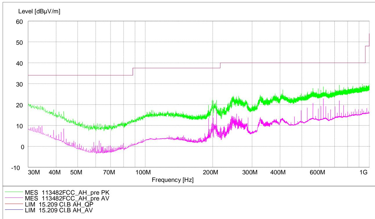
In this case it was not necessary to carry out subsequent measurements because at no frequency a value exceed the qualify limit.
