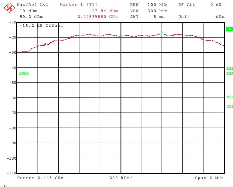
113482 .wmf: Power spectral density (radiated) (operation mode 3):
