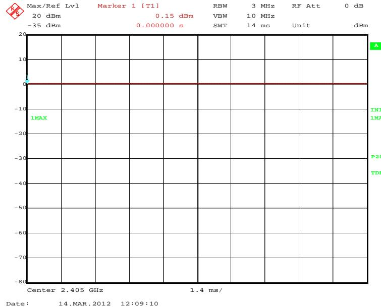
113482\_17.wmf: Effective isotropic radiated power (EIRP) (operation mode 2):
