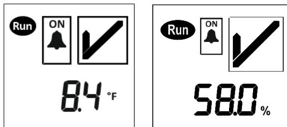
Users who want the benefit of pausing the alarming (e.g. while refilling the liquid nitrogen or while cleaning the refrigerator), can do so by pressing the "Alarming OFF" button on the device. In this case, the display shows the current temperature value (bottom, if configured), alarm indicator (top right, if configured), logging indicator (top left) and the "Alarming OFF" status (top center). LIBERO CH also shows humidity value by pressing any button (bottom, if configured).
