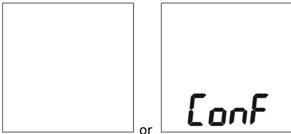
After the device has been configured, the device can be started by pressing the "Start" button for 3 seconds. The **start mode** is indicated on the display. In addition to starting the device, it can also be reconfigured from the start mode. The device is automatically recognized in liberoCONFIG.
