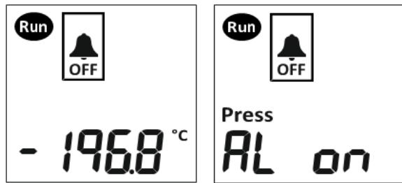
From the measuring mode, without configured "Alarming ON/OFF" function or from the measuring mode with status "Alarming OFF," the device can be stopped by pressing the "Stop" button for 3 seconds.
