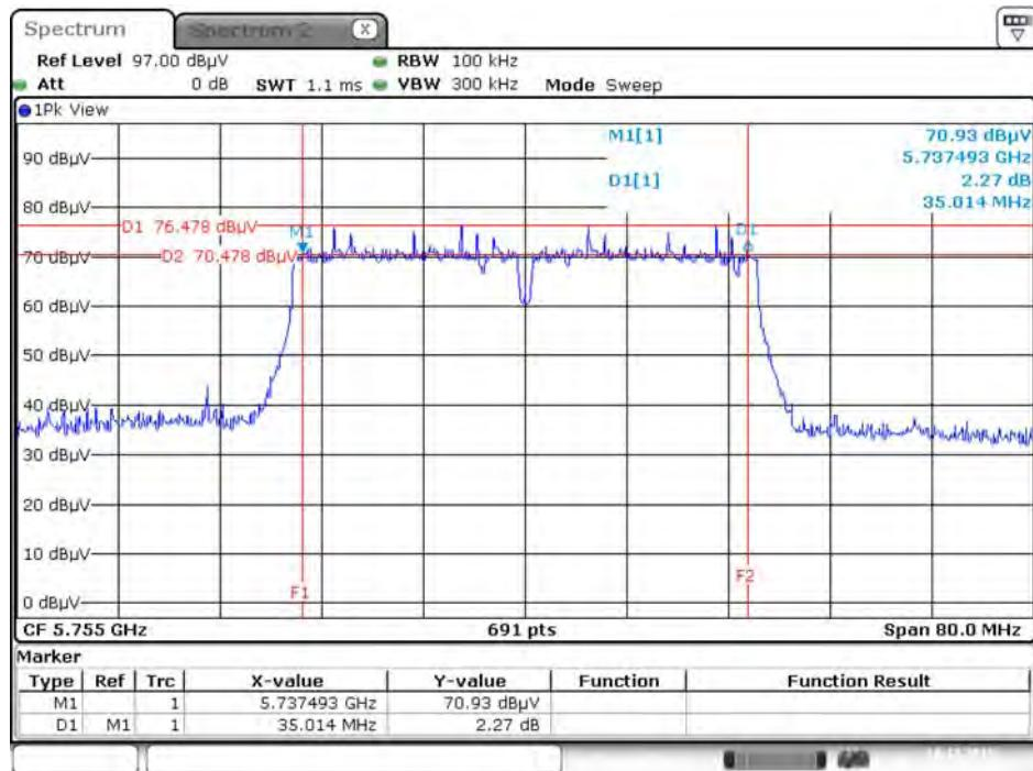
**6 dB Bandwidth Plot on Configuration IEEE 802.11ac MCS0/Nss1 VHT80 / Ant. 1 + Ant. 2 / 5775 MHz**
