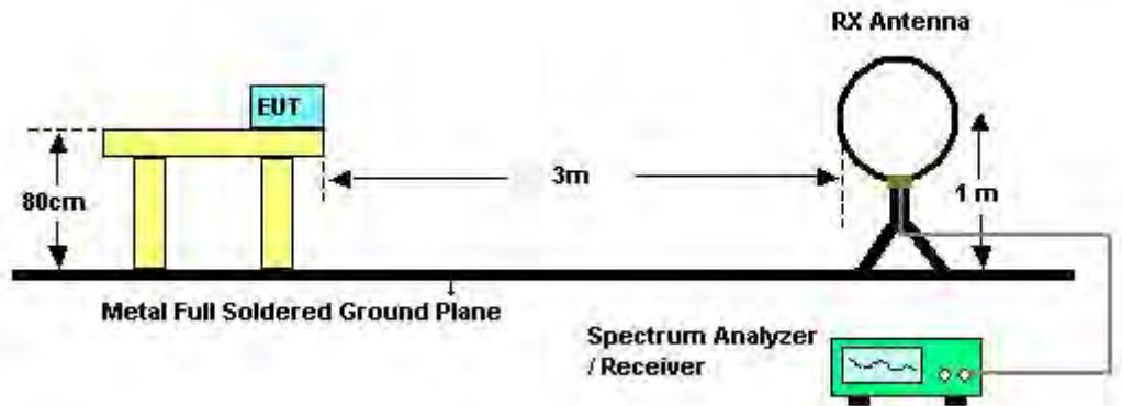
For Radiated Emissions: 30MHz~1GHz
