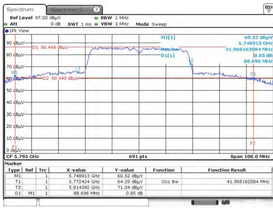
**26dB Bandwidth and 99% Occupied Bandwidth Plot on Configuration IEEE 802.11ac MCS0/Nss1 VHT80 / Ant. 1 + Ant. 2 / 5210 MHz**
