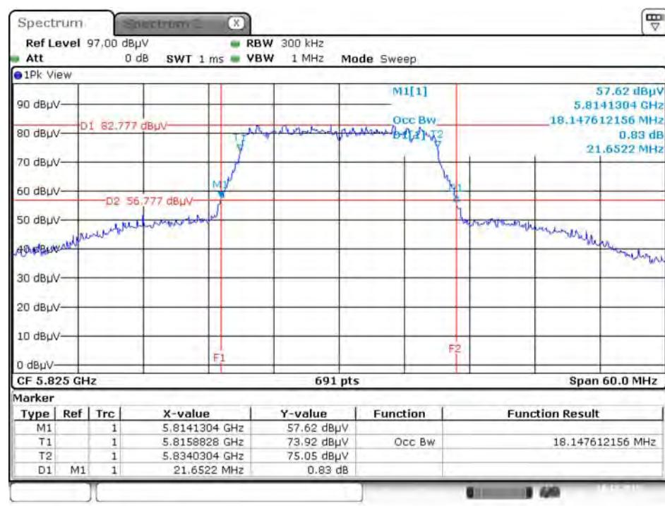
**26dB Bandwidth and 99% Occupied Bandwidth Plot on Configuration IEEE 802.11ac MCS0/Nss1 VHT40 /
