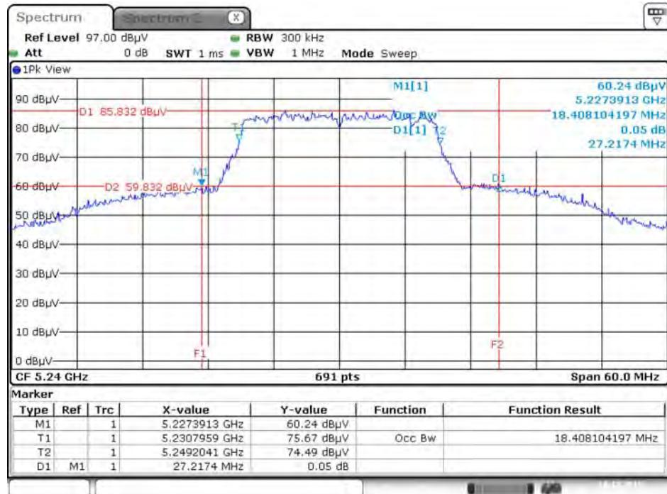
**26dB Bandwidth and 99% Occupied Bandwidth Plot on Configuration IEEE 802.11ac MCS0/Nss1 VHT20 /
