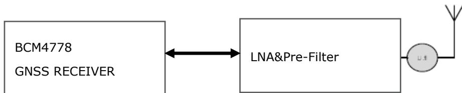
The GNSS receiver can track GPS, GA Galileo
