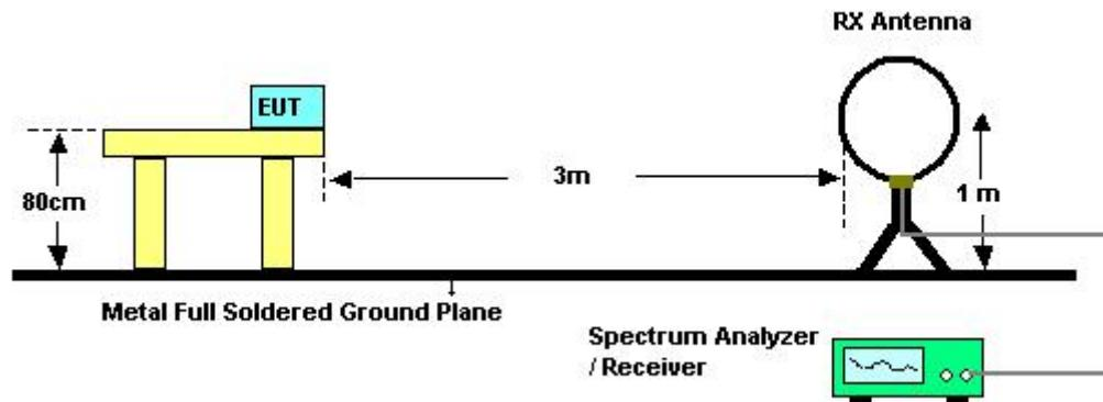
For Radiated Emissions: 30MHz~1GHz
