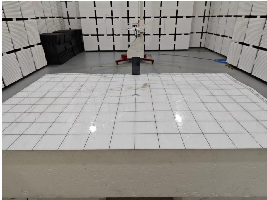
**Set-up for Radiated Emission (RE), Above 1GHz**
