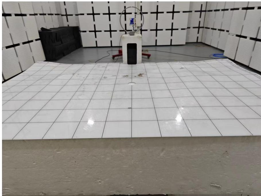
**Set-up for Radiated Emission (RE), Below 1GHz**
