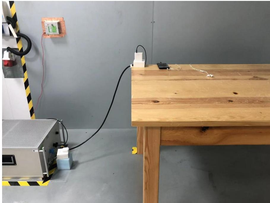
**Set-up for Radiated Emission (RE), Below30MHz**
