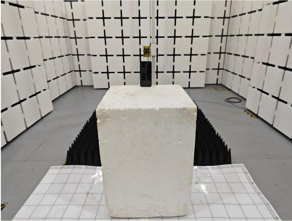
Set-up for Radiated Emission (RE), Above 1GHz
