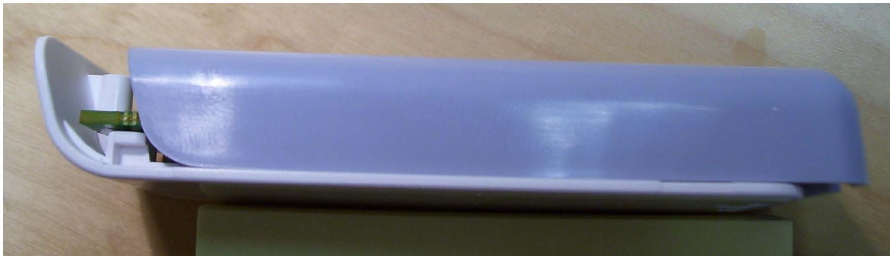
At assembly, rear housing is slightly offset and then slid forward to engage hooks
