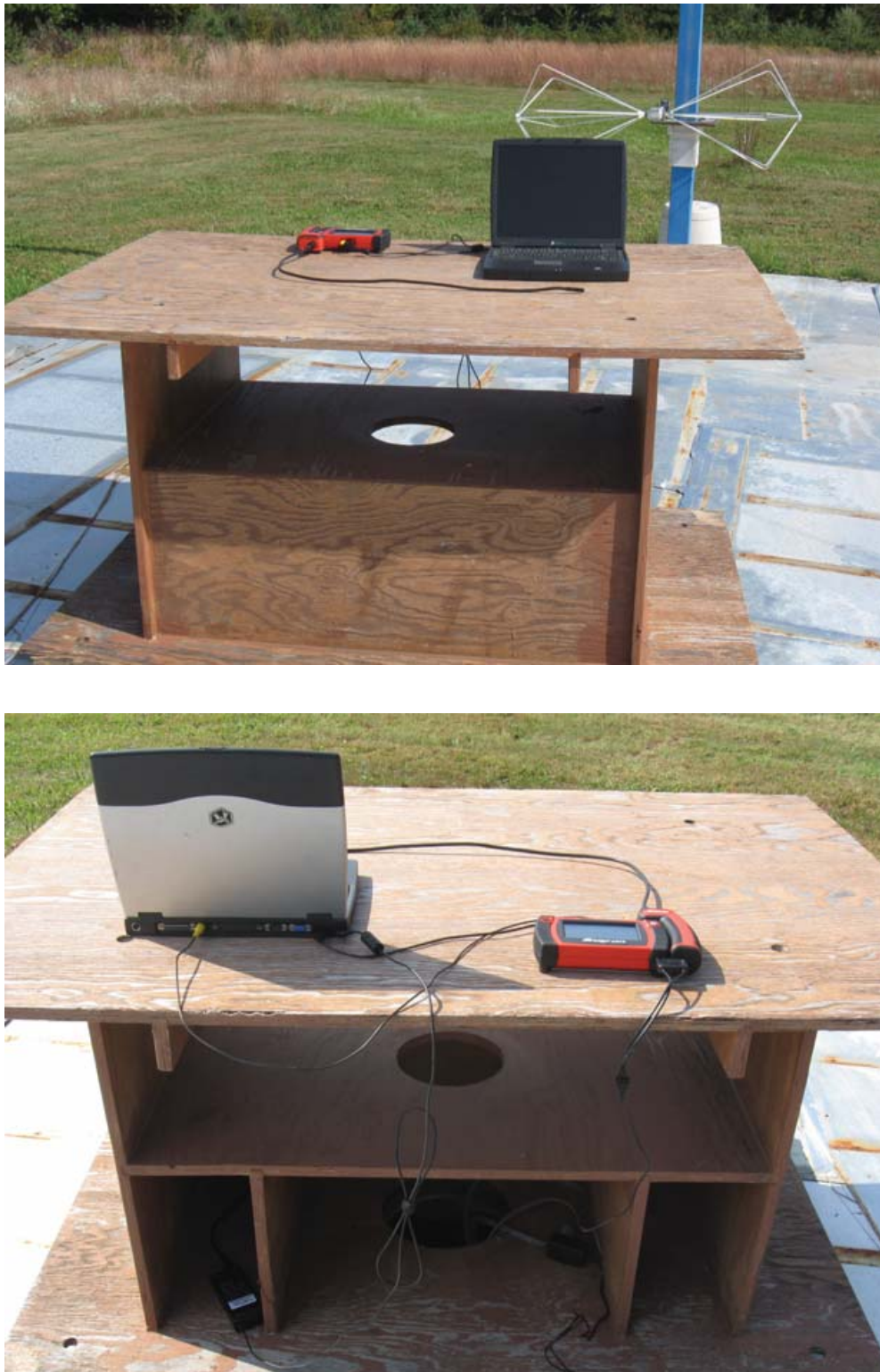
Figure 4: Radiated Emissions Test Setup Photograph(s).
