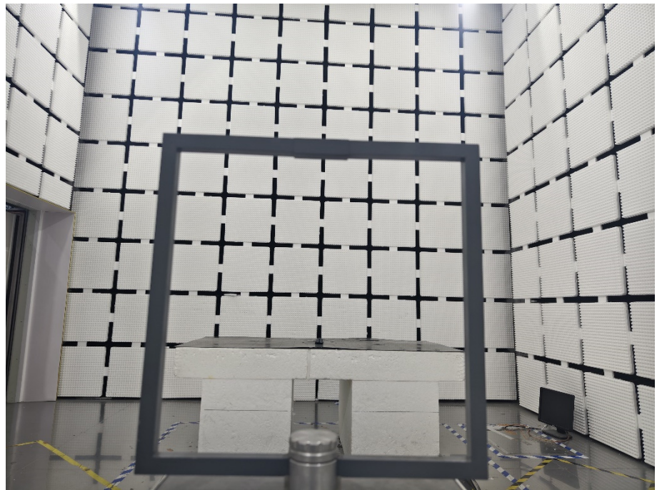
Radiation Emission Test Setup (Below 30MHz)
