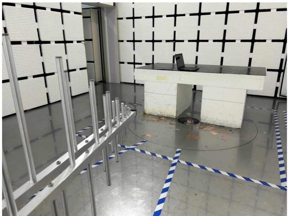
Radiation Emission Test Setup (30MHz to 1GHz)
