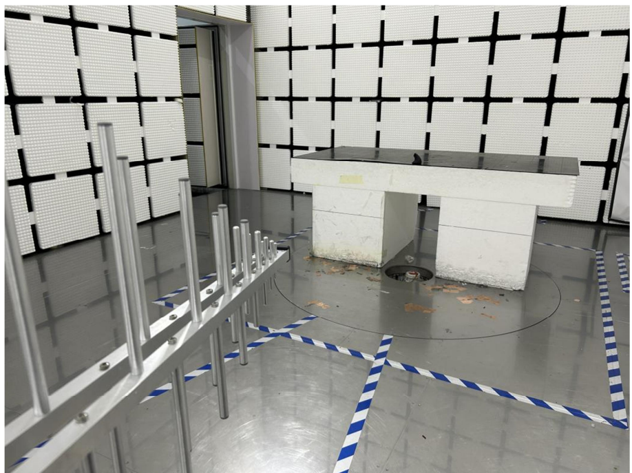
Radiation Emission Test Setup (30MHz to 1GHz)
