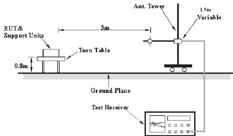
The deactivation test was performed in the 3 meters chamber test site, using the setup accordance with the ANSI C63.10- 2013. The specification used was the FCC 15.231(e) limits.
