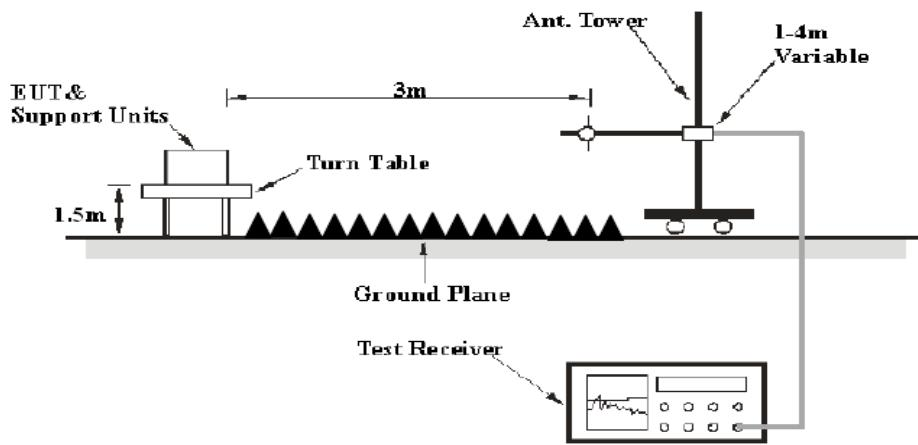
The radiated emission tests were performed in the 3-meter chamber a test site, using the setup accordance with the ANSI C63.10-2013. The specification used was the FCC Part Subpart C limits.
