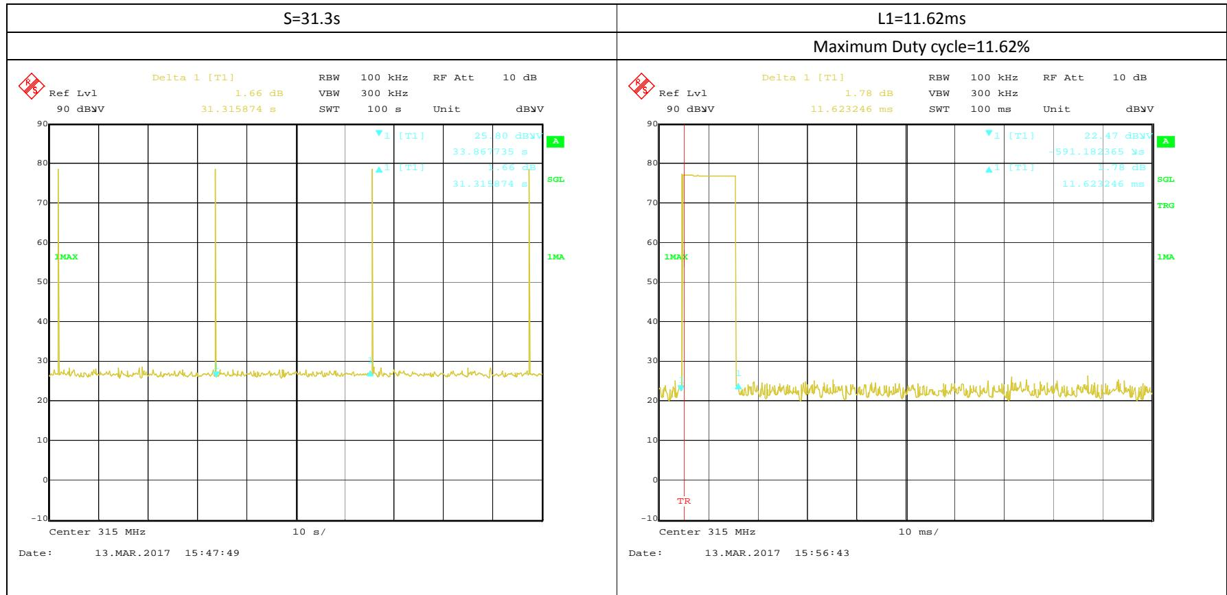
Note: The accuracy of the measurement equipment (R & S Signal Analyzer, Model Number: FSIQ26) is 1% of the sweep time. The plot on the left only shows the separation between each L1. Thus, the markers were roughly placed. This device's duty cycle was measured and determined in the plot on the right. The tolerance between measured L1 and theoretical L1 is within the measurement equipment accuracy.
