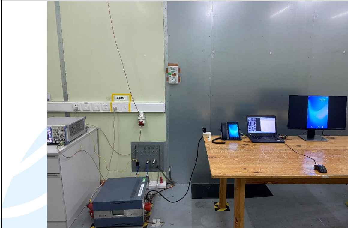
Conducted Emission Test Setup
