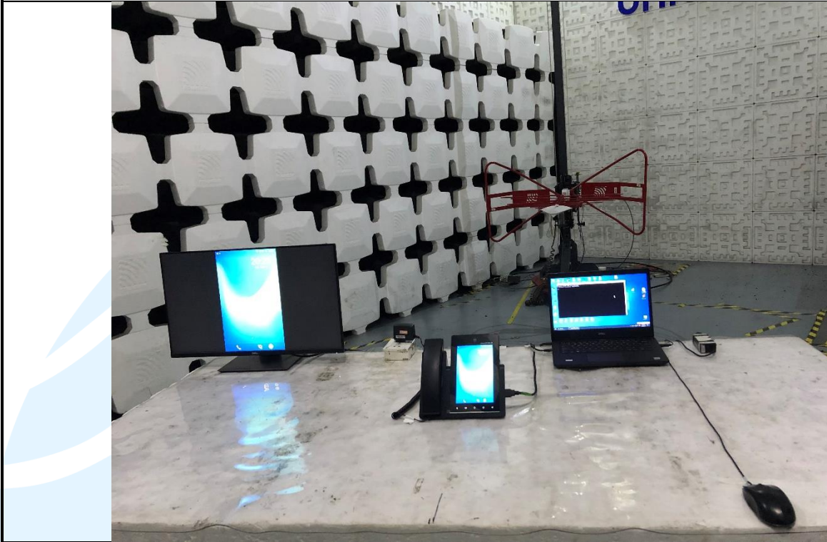
Radiated emission Test Setup (30 MHz~1 GHz)
