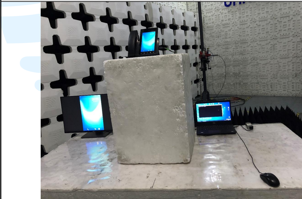
Radiated emission Test Setup (Above 1 GHz)
