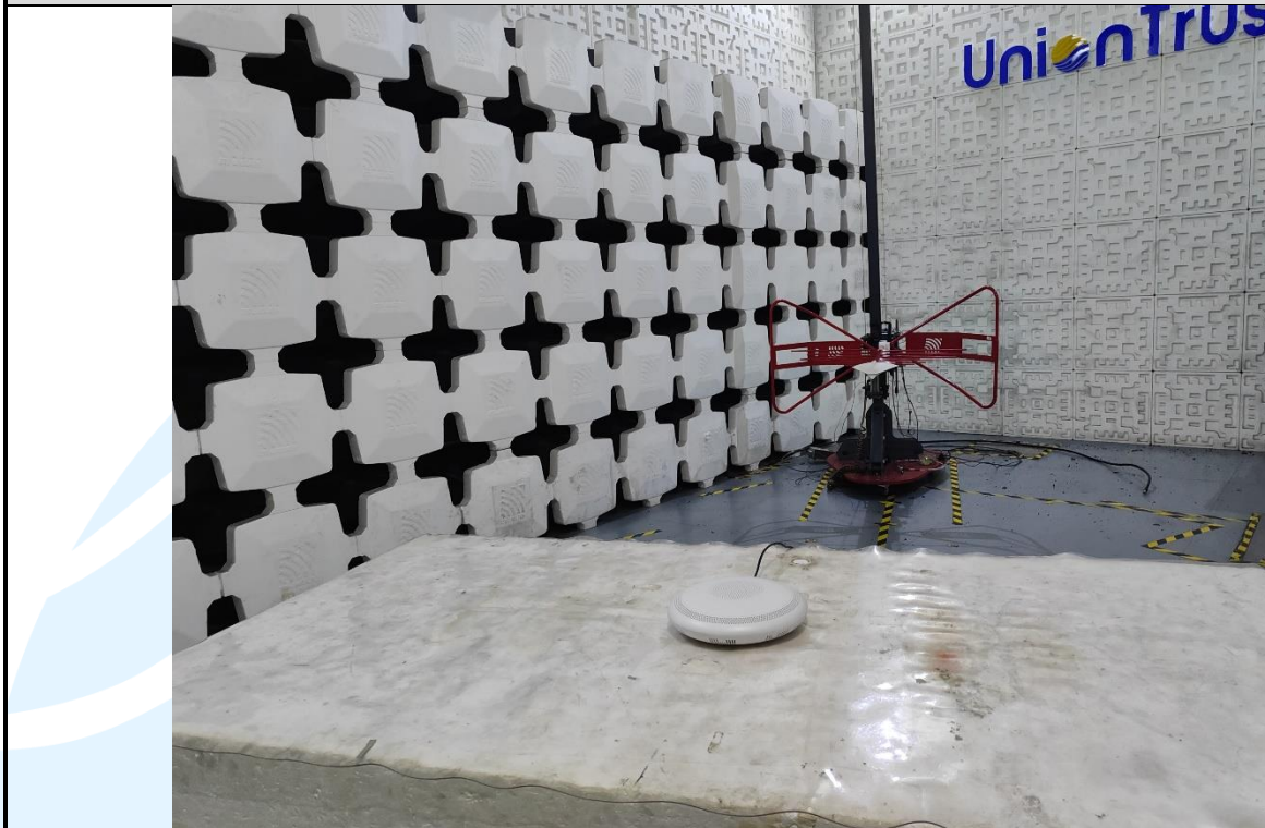
Radiated emission Test Setup (30 MHz~1 GHz)
