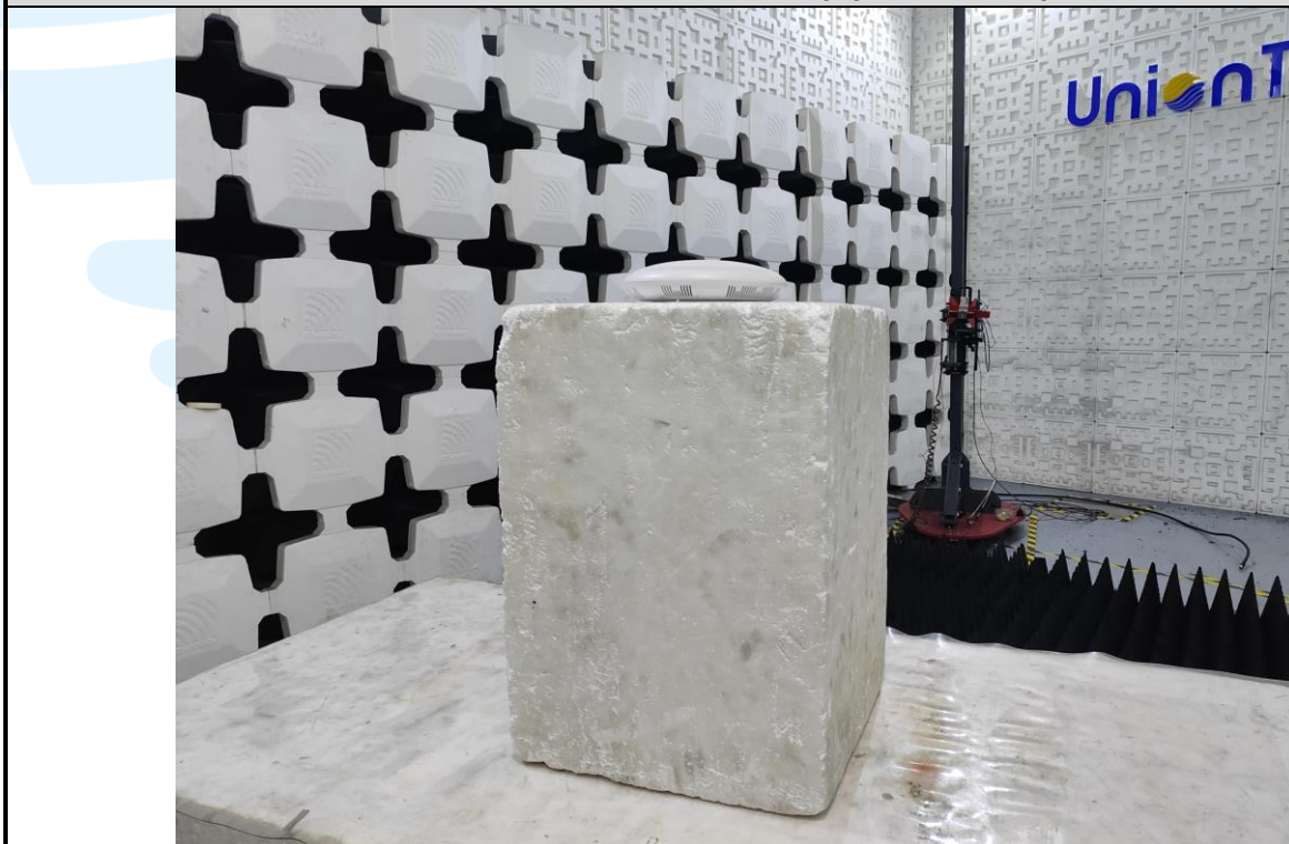
Radiated emission Test Setup (Above 1 GHz)
