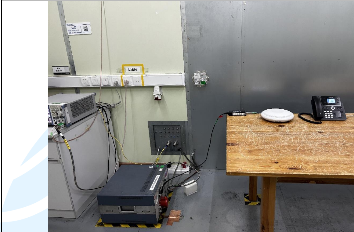
Conducted Emission Test Setup
