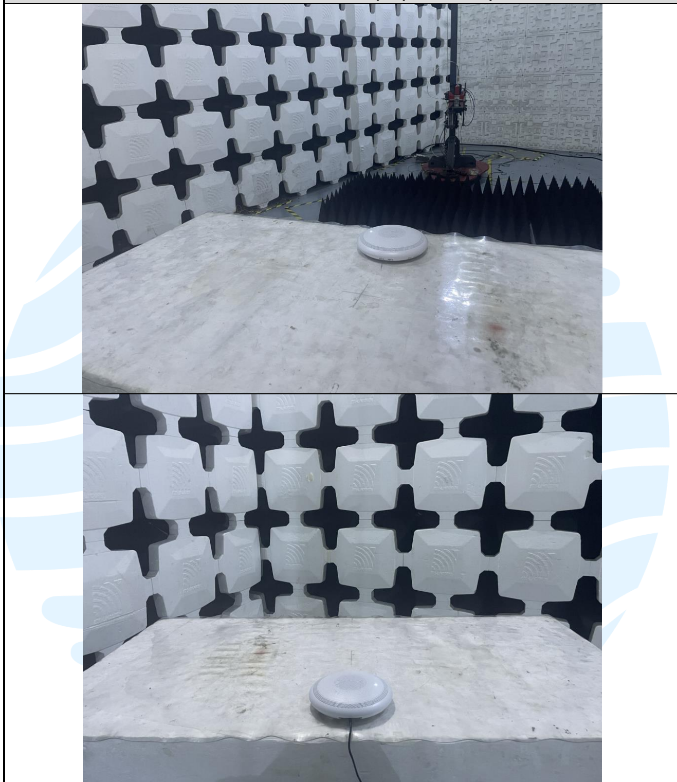
Radiated emission Test Setup-2 (Above 1 GHz)
