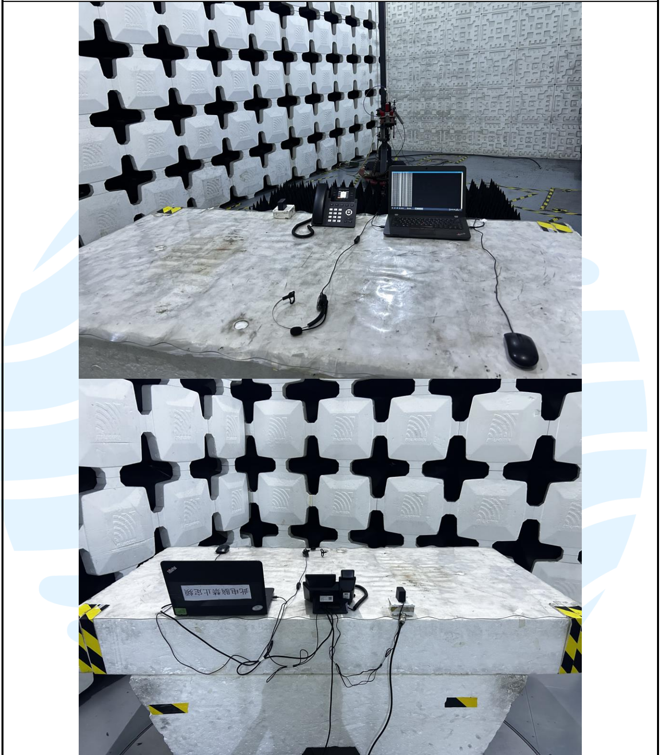
Radiated emission Test Setup-2 (Above 1 GHz)
