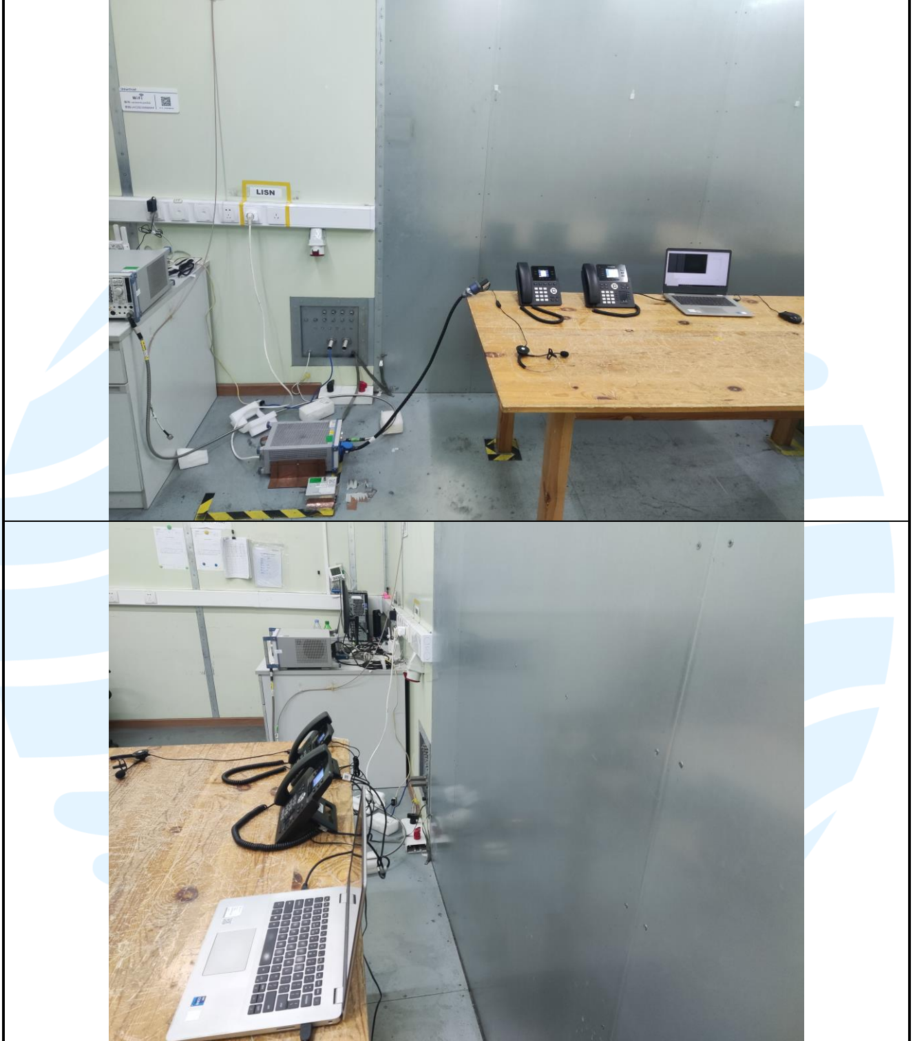
Conducted Emission Test Setup-3
