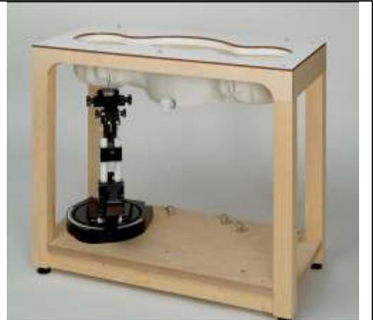
**Fig. 8.7 Photo of SAM Twin Phantom**
