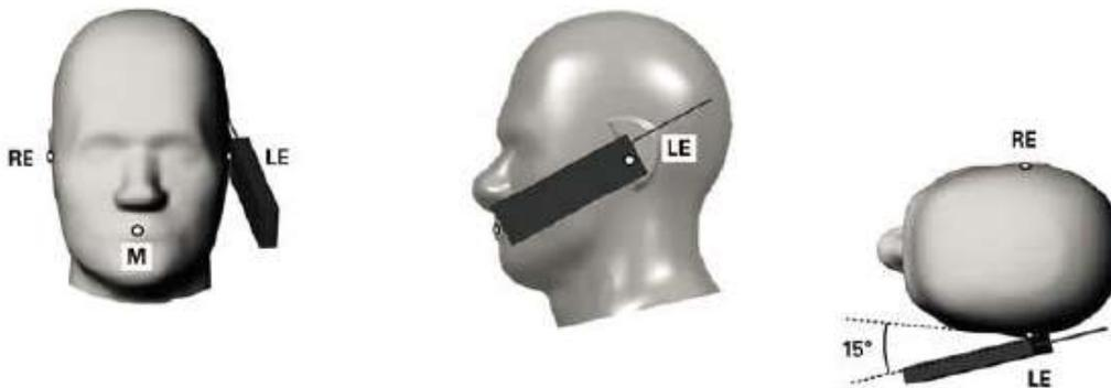
Fig.11.4 Illustration for Tilted Position
