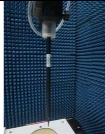
Fig. 8.2 Photo of E-Field Probe
