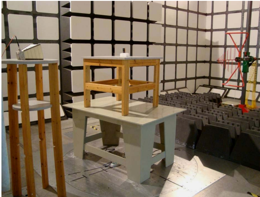
Below 1 GHz: Radiated Emissions - Rear View
