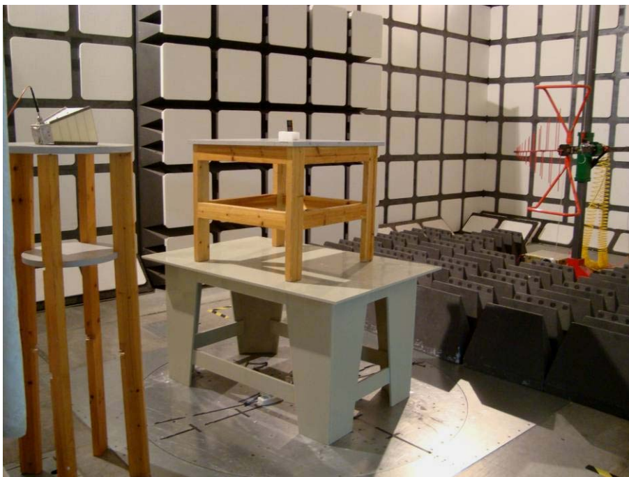
Below 1 GHz: Radiated Emissions - Rear View
