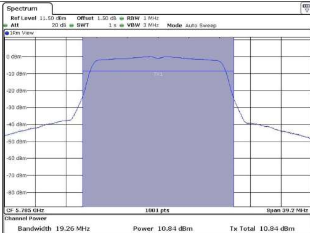
Low Channel @ 5.745 MHz (26 dB Bandwidth)
