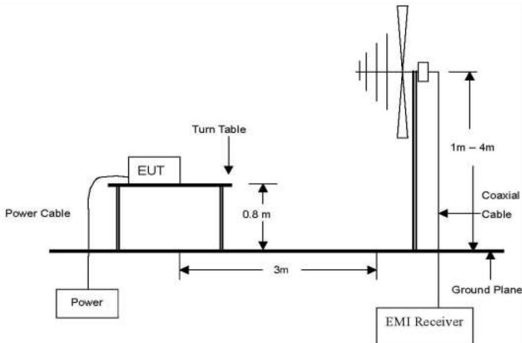
The diagram below shows the test setup that is utilized to make the measurements for emission .The spurious emissions were investigated from 1 GHz to the 10th harmonic of the highest fundamental frequency or 40 GHz, whichever is lower.
