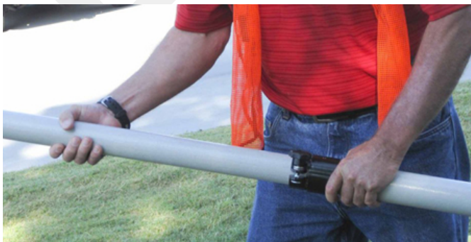
Figure 4-32 Inserting the Electronics Carrier into the Mast
