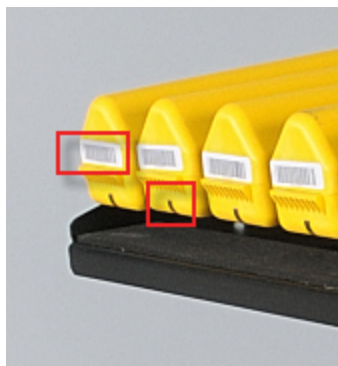
Figure 7-3 Serial Number Label and LED Indicator
