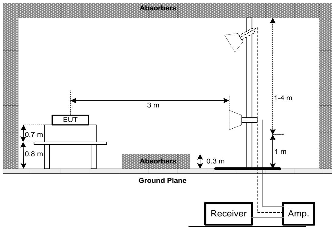
(C) For Radiated Emissions Below 30MHz
