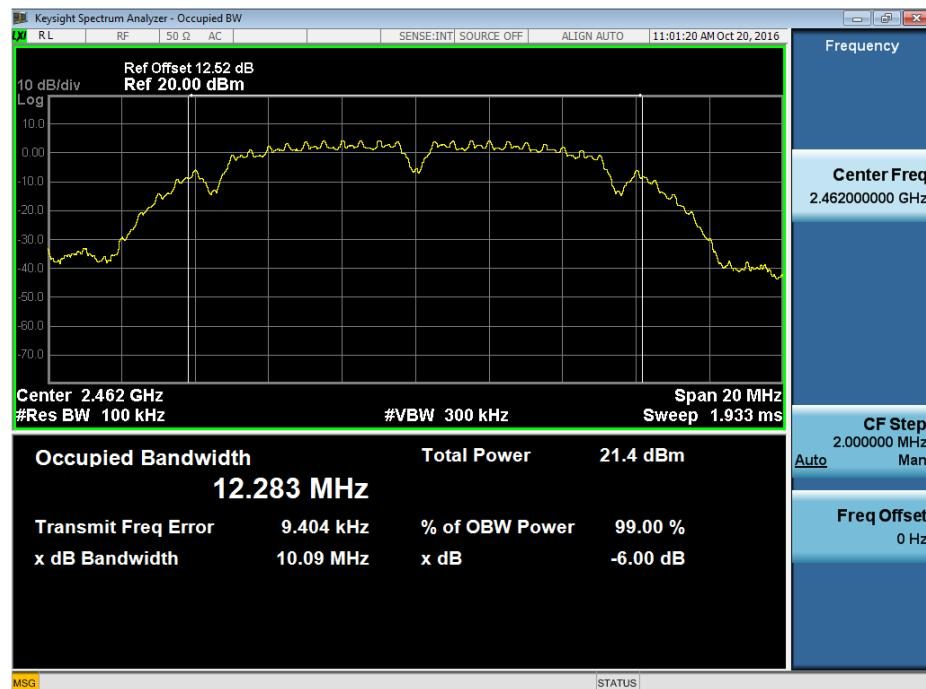
**Test Mode : TX B Mode\_CH01/06/11\_ANT 2**
