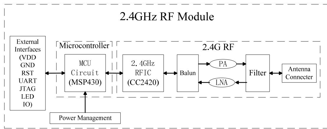
SIA2420 integrates a low noise amplifier (LNA) and a power amplifier (PA).
