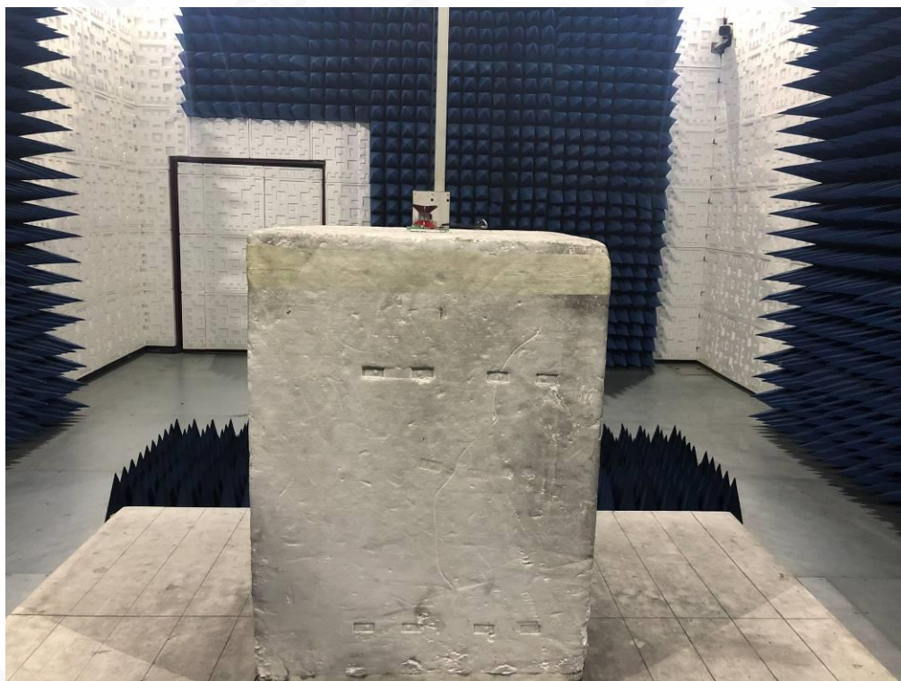
FCC RADIATED EMISSION TEST SETUP ABOVE 1GHZ
