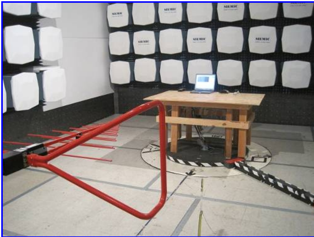
Front View of Radiated Emission Test Setup
