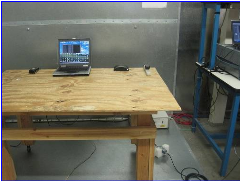
Front View of Conducted Emission Test Setup
