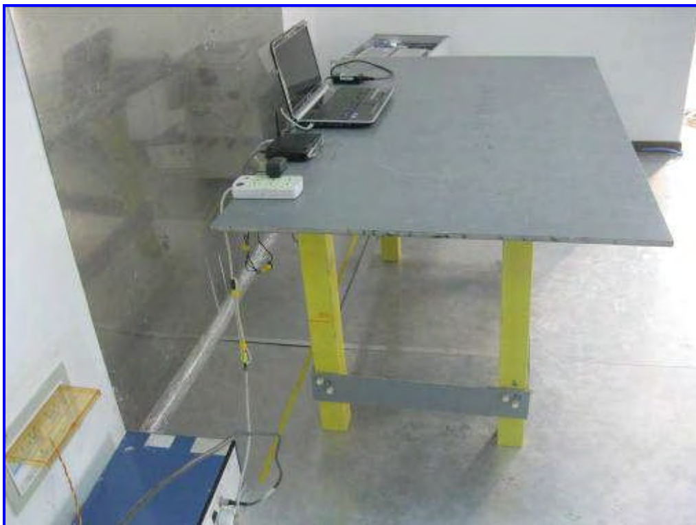
Side View of Conducted Emission Test Setup
