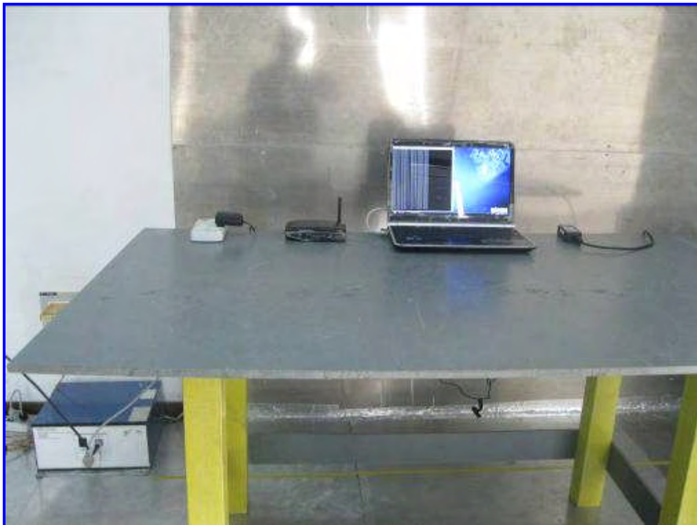
Front View of Conducted Emission Test Setup
