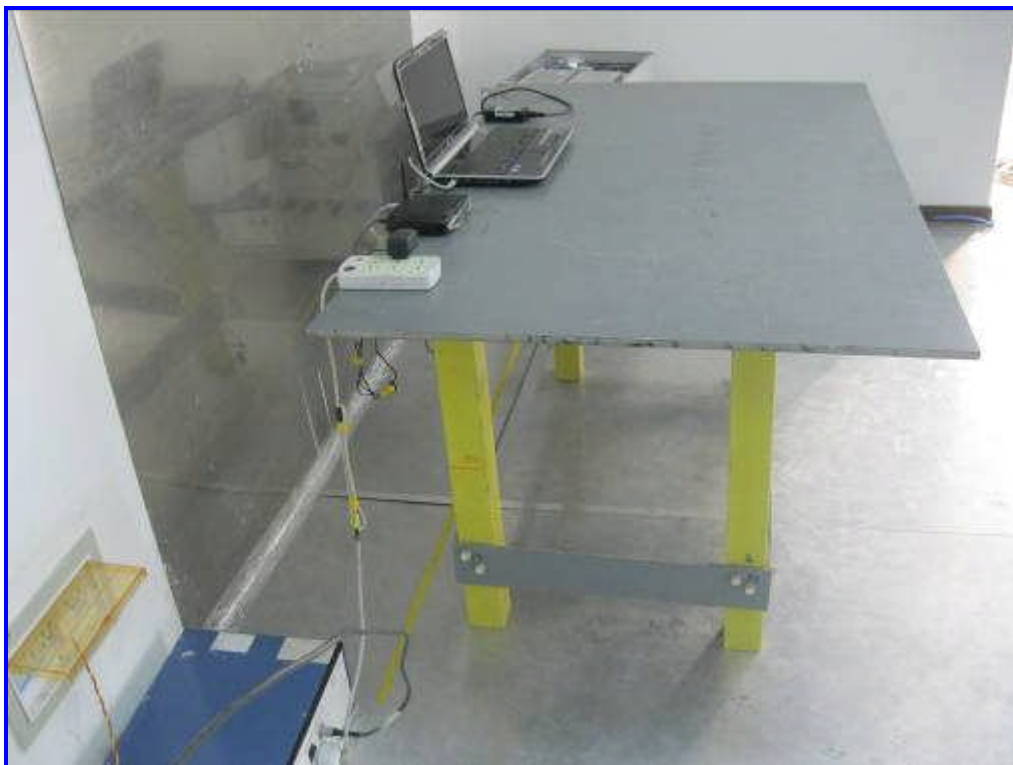
Side View of Conducted Emission Test Setup
