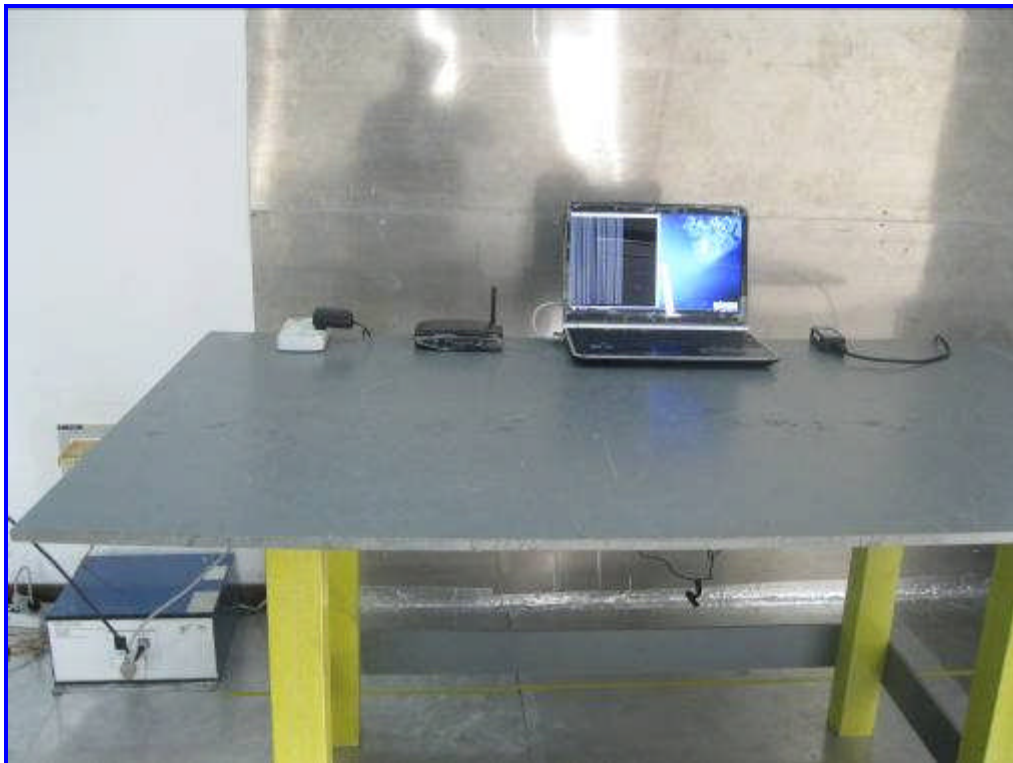
Front View of Conducted Emission Test Setup
