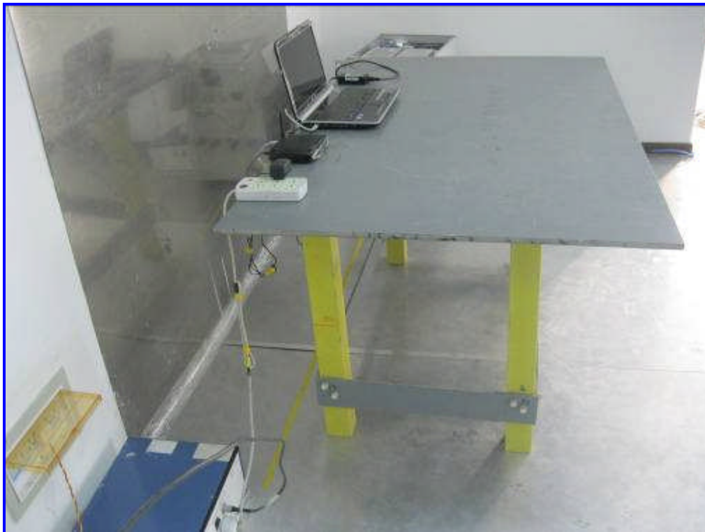
Side View of Conducted Emissions Test Setup
