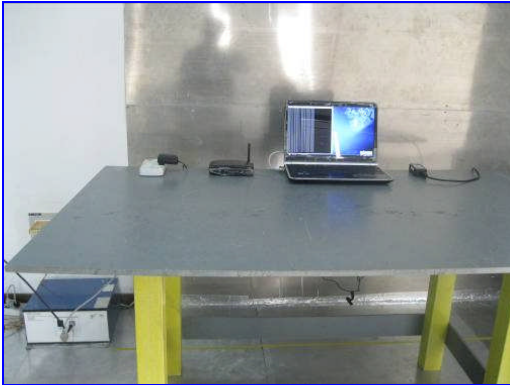
Front View of Conducted Emissions Test Setup
