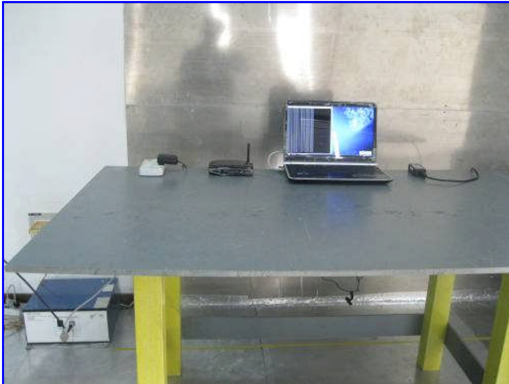
Front View of Conducted Emissions Test Setup
