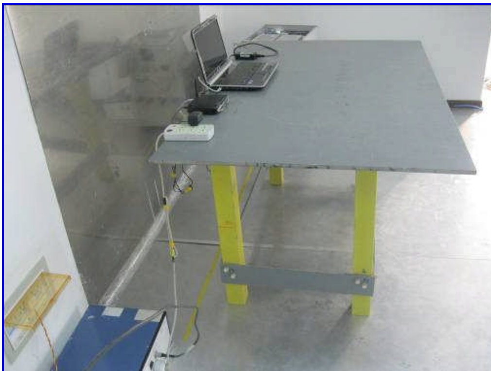
Side View of Conducted Emissions Test Setup
