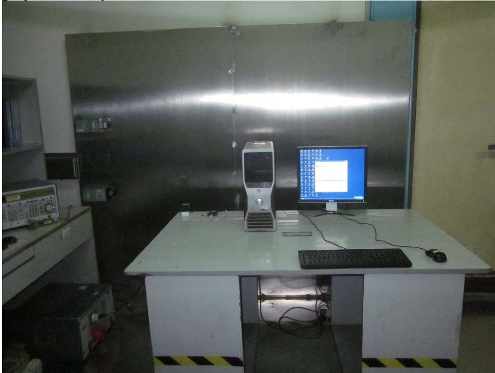
Photograph 2: Set-up for Spurious Emissions 30MHz – 1GHz
