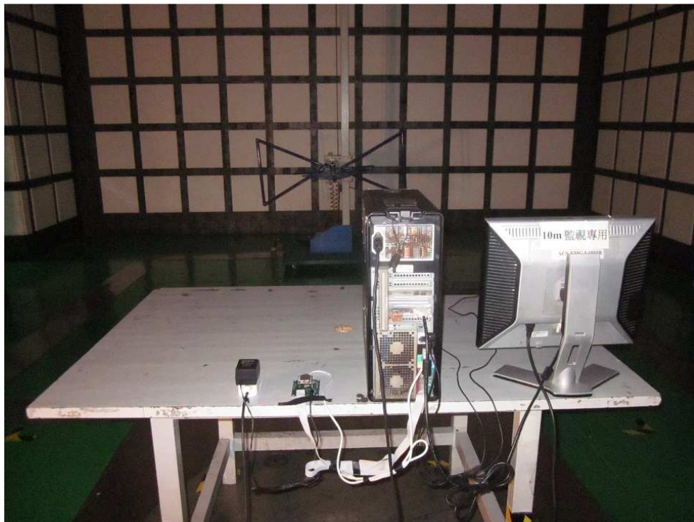
Photograph 2: Set-up for Spurious Emissions 30MHz – 1GHz
