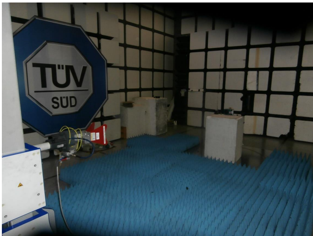
Figure 32 – Test Setup - Radiated Emissions – 1 GHz to 18 GHz
