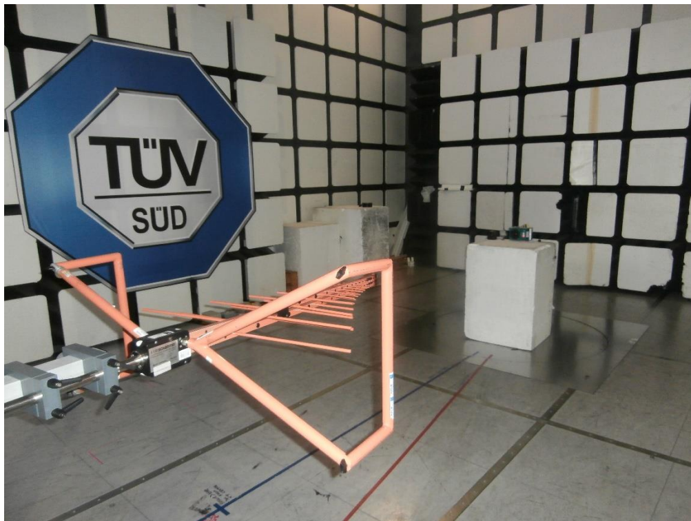
Figure 31 – Test Setup - Radiated Emissions – 30 MHz to 1 GHz
