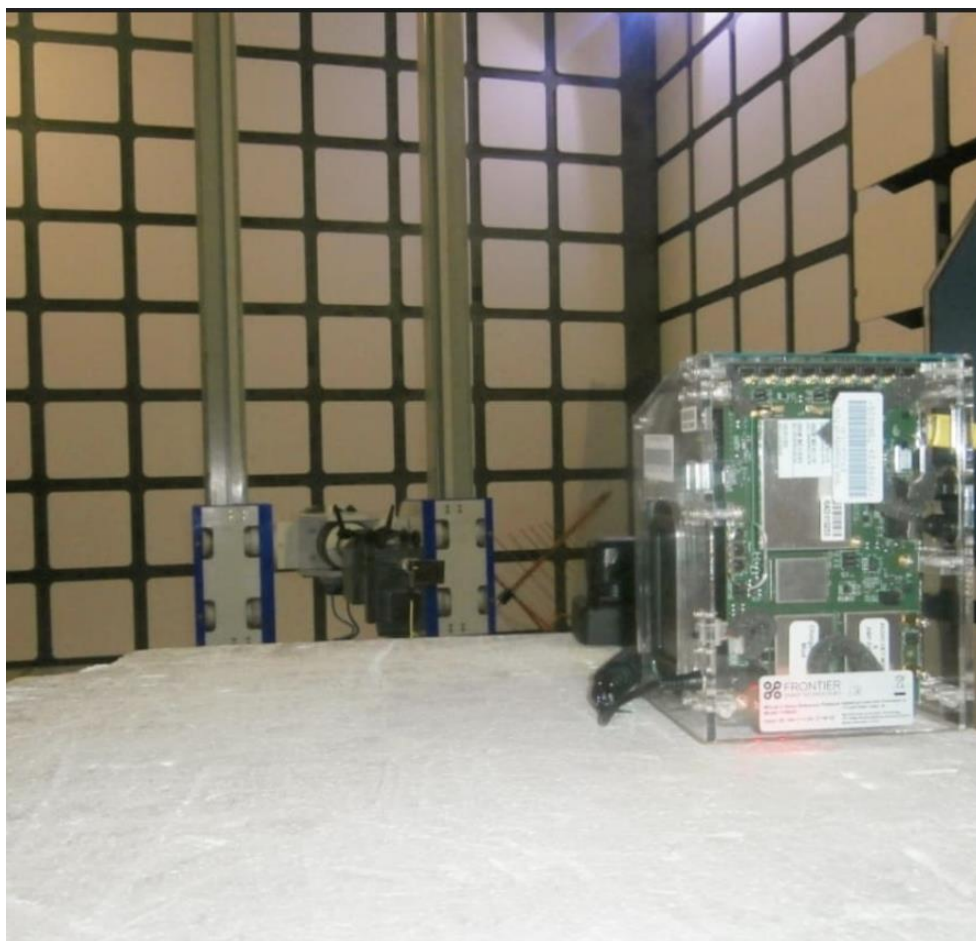
Figure 33 – Test Setup - Radiated Emissions – 18 GHz to 30 GHz
