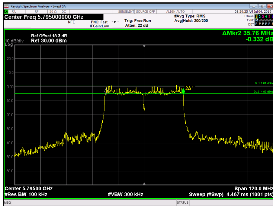
Figure 363 - 5795 MHz - 6 dB DTS Bandwidth – Worst-case Antenna Port
