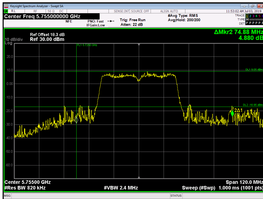
Figure 361 - 5755 MHz - 26 dB Emission Bandwidth – Worst-case Antenna Port
