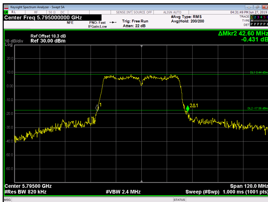
Figure 307 - 5795 MHz - 26 dB Emission Bandwidth – SISO – Antenna Port 0
