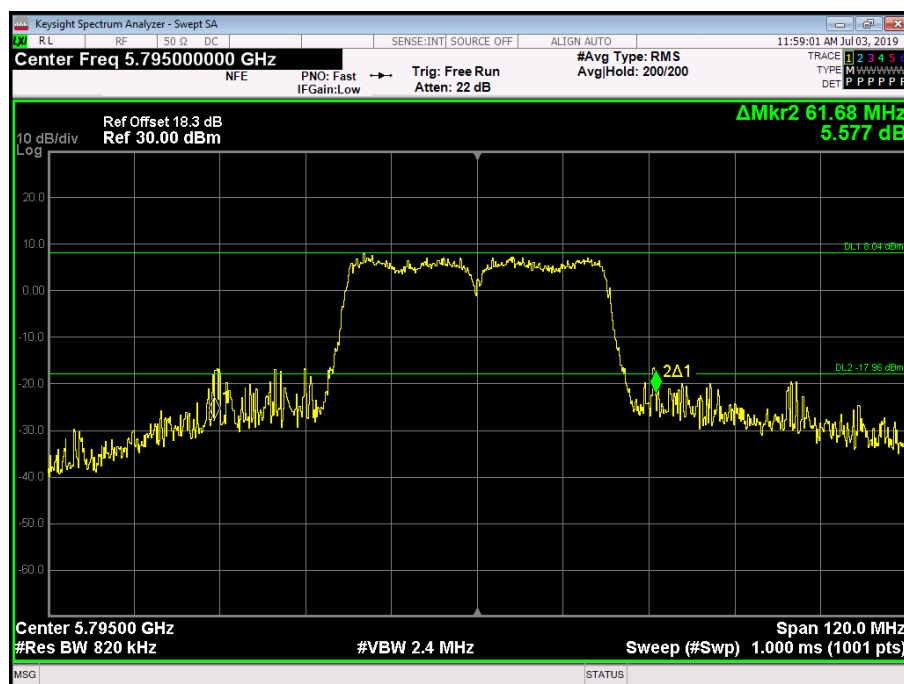
Figure 364 - 5795 MHz - 26 dB Emission Bandwidth – Worst-case Antenna Port
