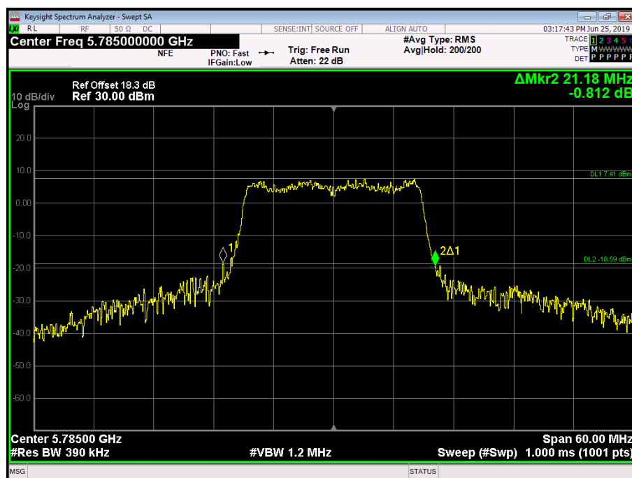
Figure 280 - 5785 MHz - 26 dB Emission Bandwidth – SISO – Antenna Port 0
