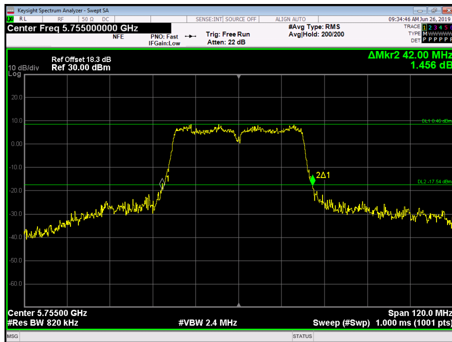
Figure 304 - 5755 MHz - 26 dB Emission Bandwidth – SISO – Antenna Port 0
