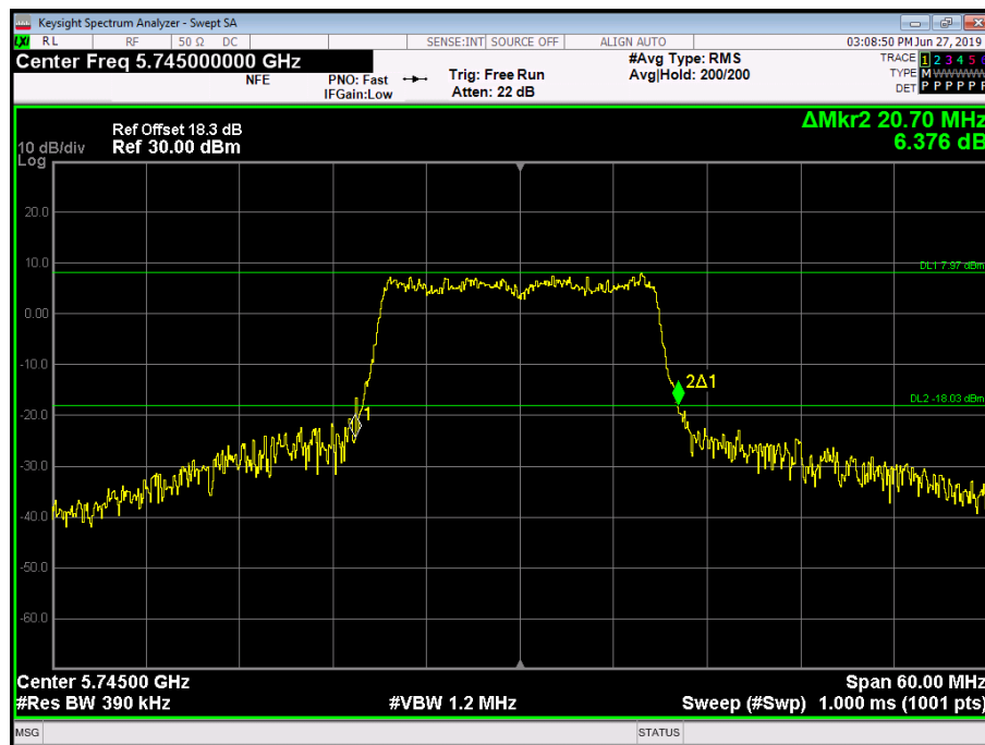
Figure 286 - 5745 MHz - 26 dB Emission Bandwidth – SISO – Antenna Port 1
