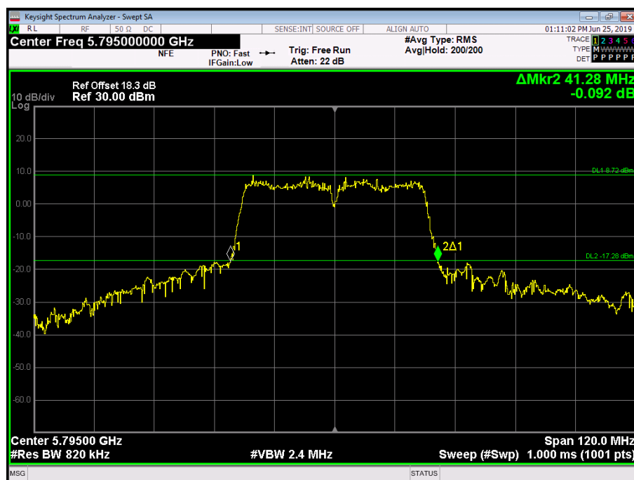
Figure 352 - 5795 MHz - 26 dB Emission Bandwidth – SISO – Antenna Port 0
