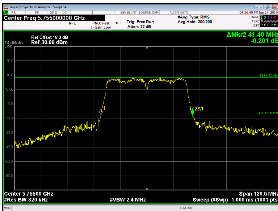
Figure 310 - 5755 MHz - 26 dB Emission Bandwidth – SISO – Antenna Port 1
