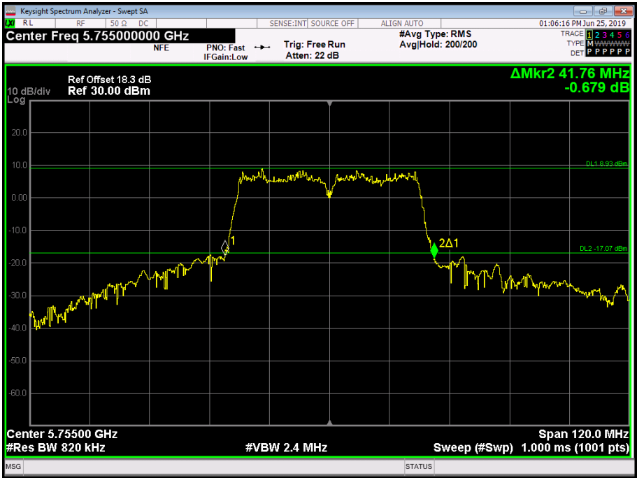
Figure 349 - 5755 MHz - 26 dB Emission Bandwidth – SISO – Antenna Port 0
