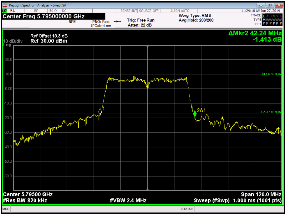
Figure 358 - 5795 MHz - 26 dB Emission Bandwidth – SISO – Antenna Port 1
