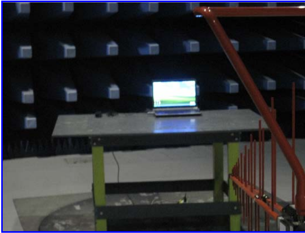
Front View of Radiated Emission Test Setup
