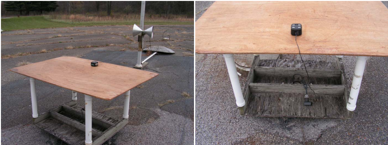
Photograph 6.4. (left) DUT on OATS, (right) Close-up on OATS (one of three axes tested)
