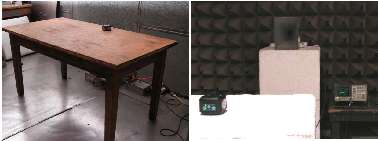
Photograph 6.5. (left) DUT on Conducted Emissions Table, (right) Indoor Setup (one of three axes tested)
