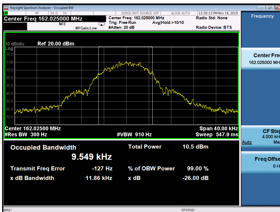
Figure 2 - 162.025 MHz Occupied Bandwidth
