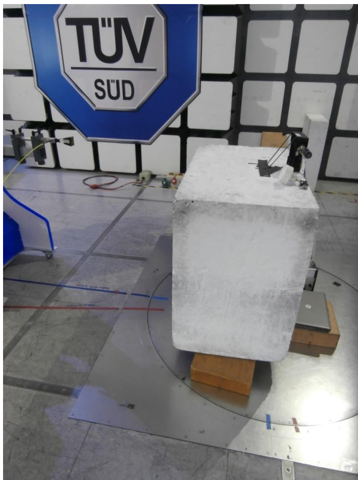
Figure 8 – Test Setup 18 GHz to 30 GHz - Z Orientation
