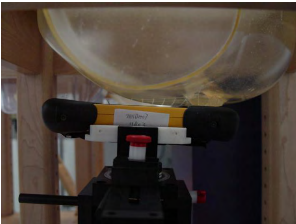
Figure B.4 EUT Right Cheek Position
