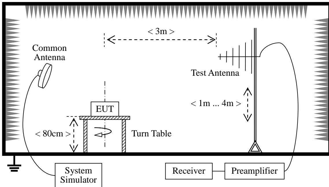
The test is performed in a 3m Semi-Anechoic Chamber; the antenna factor, cable loss and so on of the site (factors) is calculated to correct the reading. The EUT is placed on a 0.8m high insulating Turn Table, and keeps 3m away from the Test Antenna, which is mounted on a variable-height antenna master tower. The Common Antenna is used for the call between the EUT and the System Simulator (SS).
