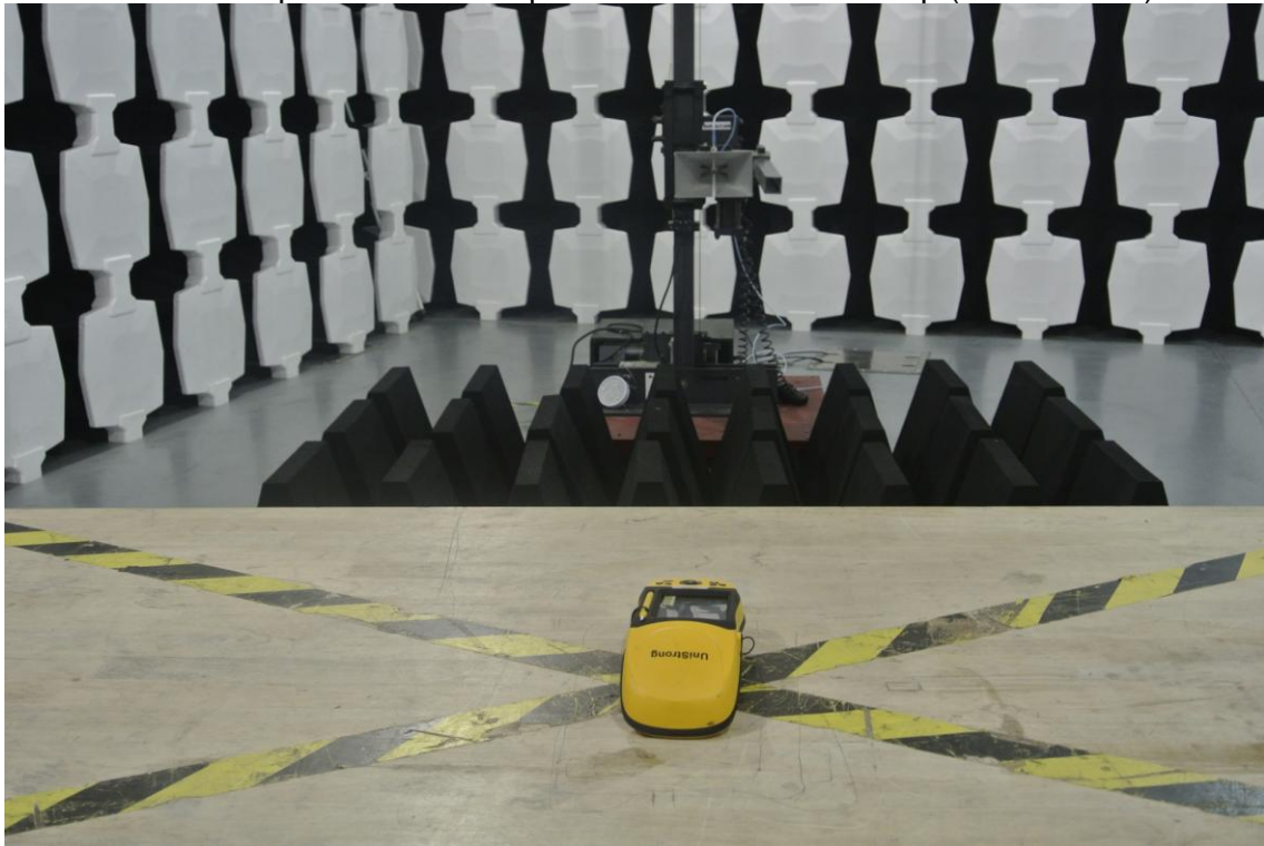
Description: Radiated Spurious Measurement Setup (Above 1GHz)
