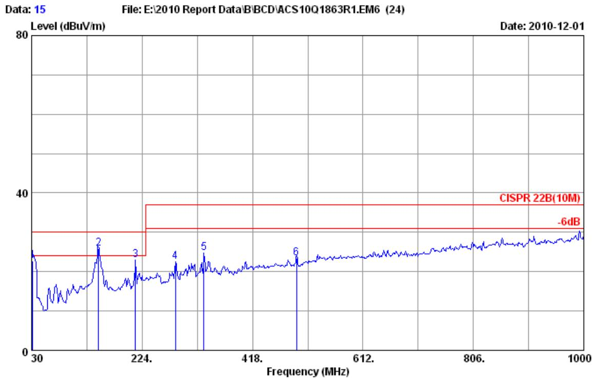
Site no. : 10m Chamber Test Site Data No. : 15
