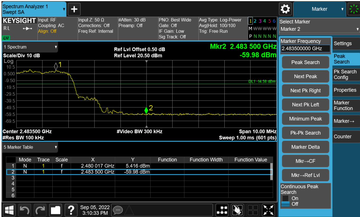
Figure 60: The plots of Conducted Spurious Emission & Authorized-band band-edge, Hopping Mode, \pi/4 -DQPSK, Conducted spurious emissions 30MHz-3GHz
