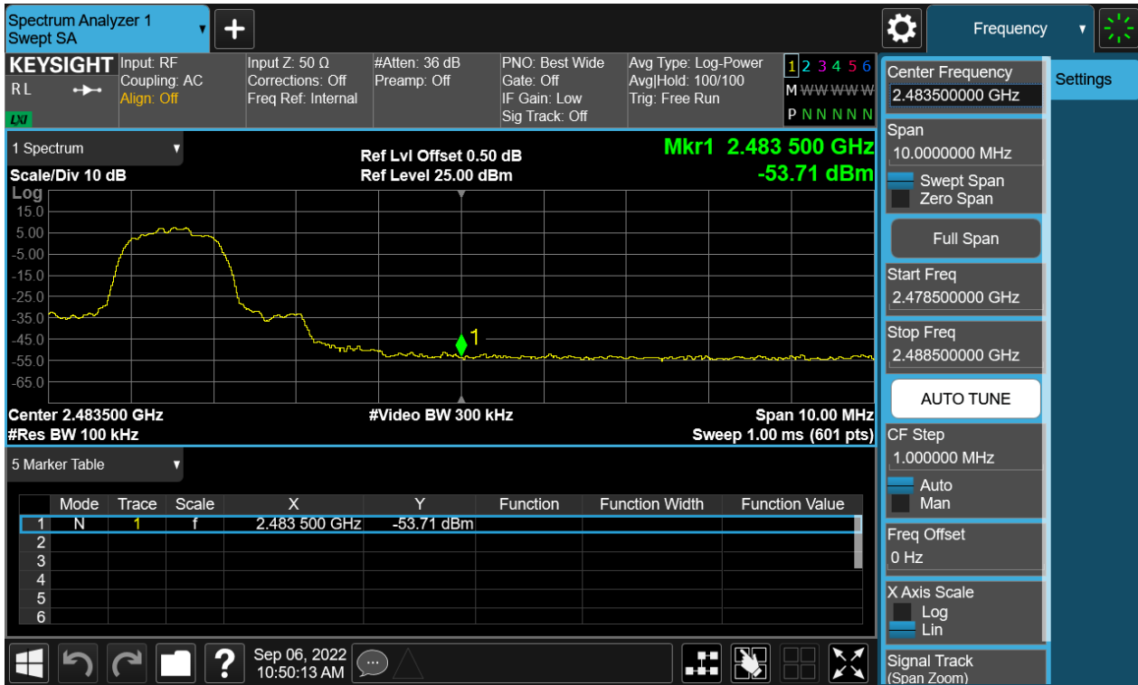
Figure 50: The plots of Conducted Spurious Emission & Authorized-band band-edge, 2480MHz, 8-DPSK Conducted spurious emissions 30MHz-3GHz
