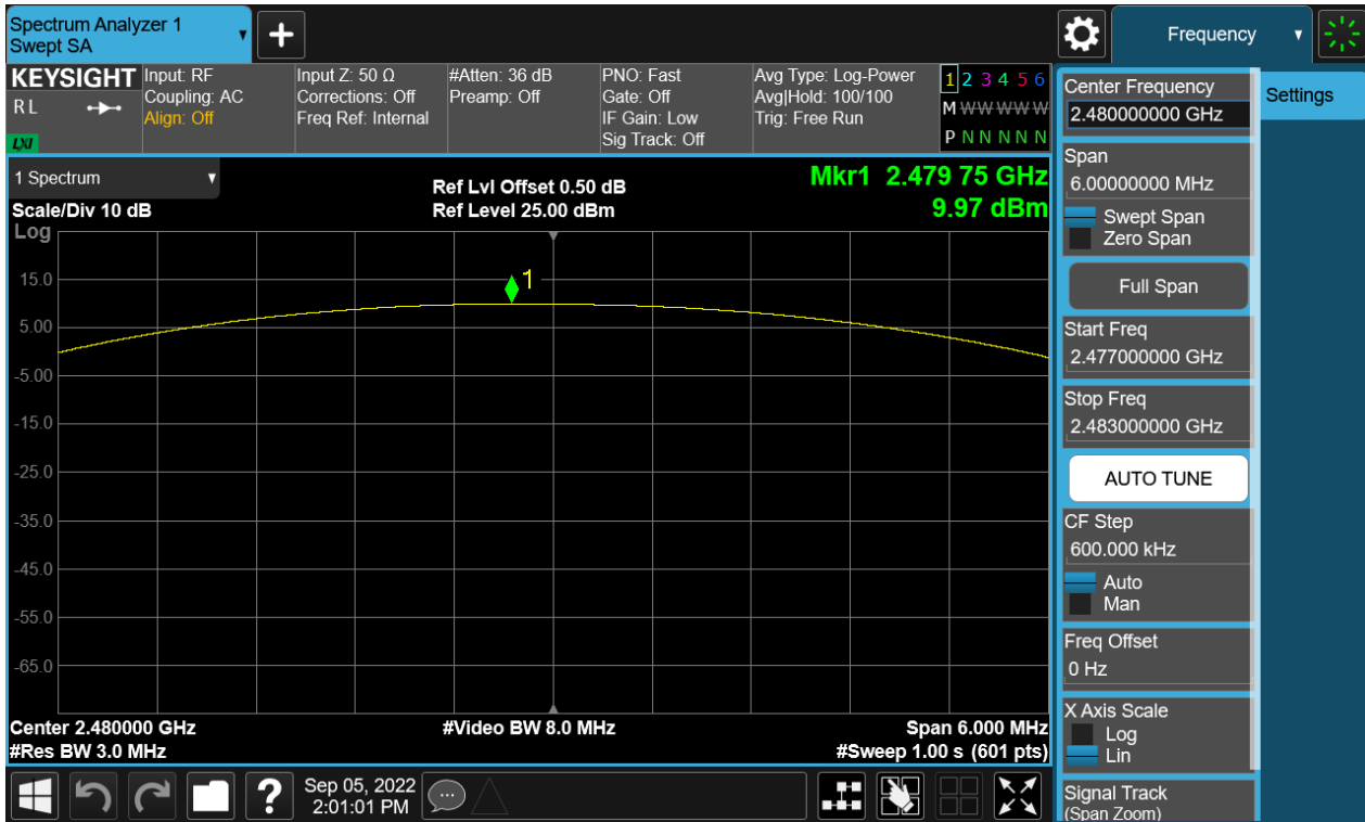
Figure 4: The plots of Maximum Conducted Peak Output Power, 2402MHz, \pi/4 -DQPSK
