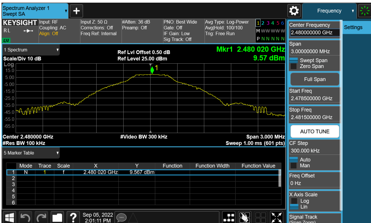
Figure 26: The plots of Conducted Spurious Emission & Authorized-band band-edge, 2480MHz, GFSK Carrier Level
