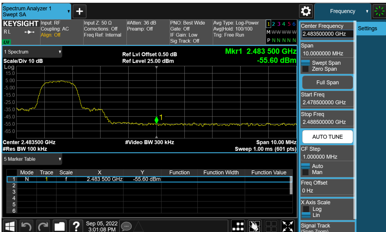
Figure 38: The plots of Conducted Spurious Emission & Authorized-band band-edge, 2480MHz, \pi/4 -DQPSK Band Edge
