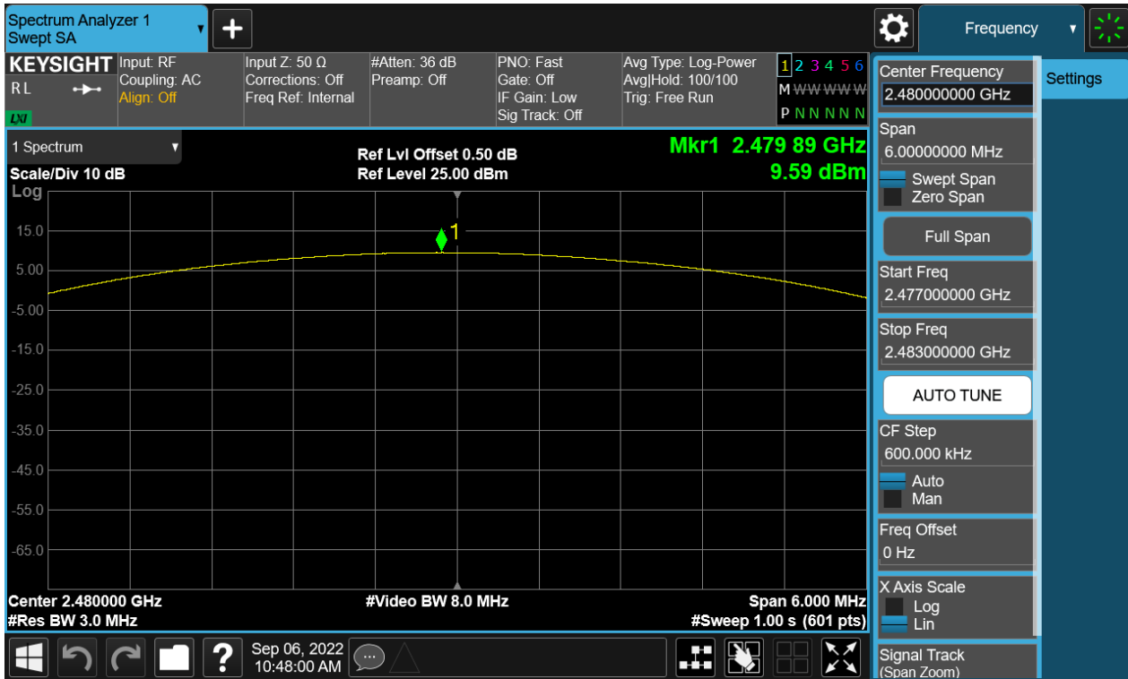
Figure 9: The plots of Maximum Conducted Peak Output Power, 2480MHz, 8-DPSK
