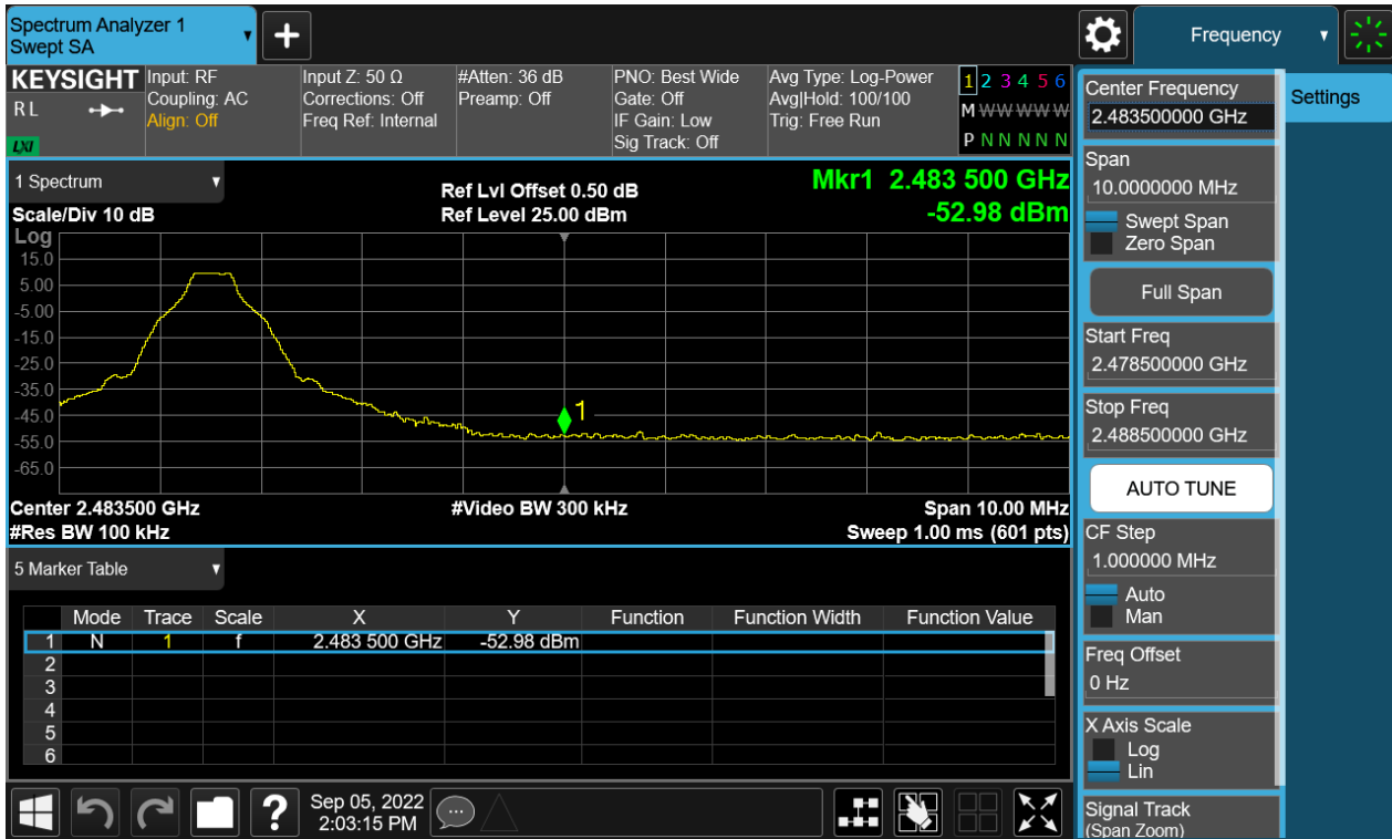
Figure 28: The plots of Conducted Spurious Emission & Authorized-band band-edge, 2480MHz, GFSK Conducted spurious emissions 30MHz-3GHz
