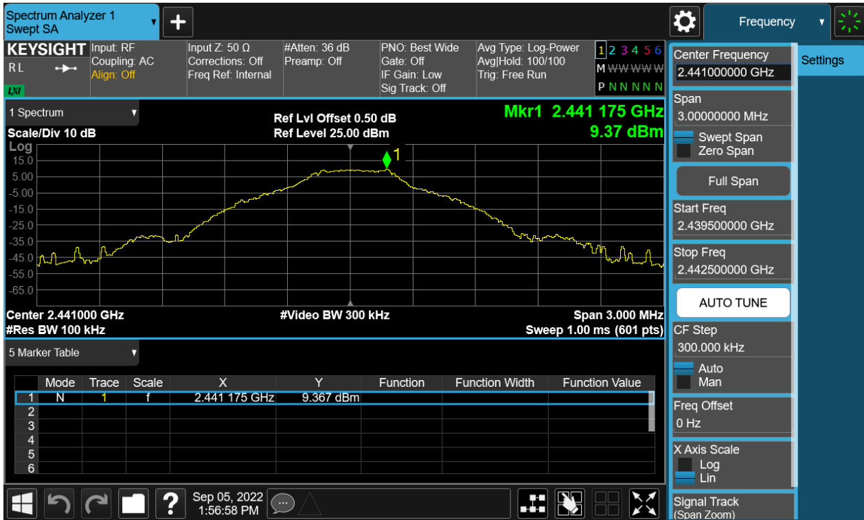
Figure 24: The plots of Conducted Spurious Emission & Authorized-band band-edge, 2441MHz, GFSK Conducted spurious emissions 30MHz-3GHz
