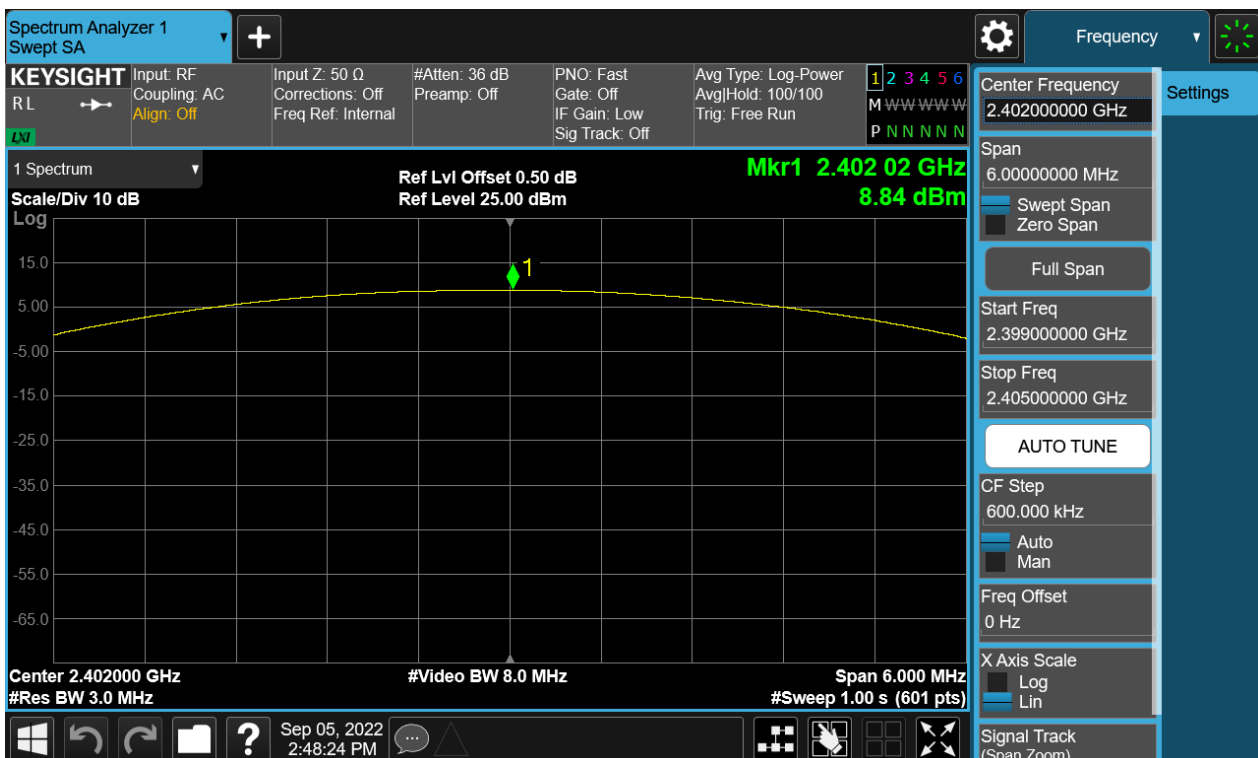
Figure 4: The plots of Maximum Conducted Peak Output Power, 2402MHz, \pi/4 -DQPSK
