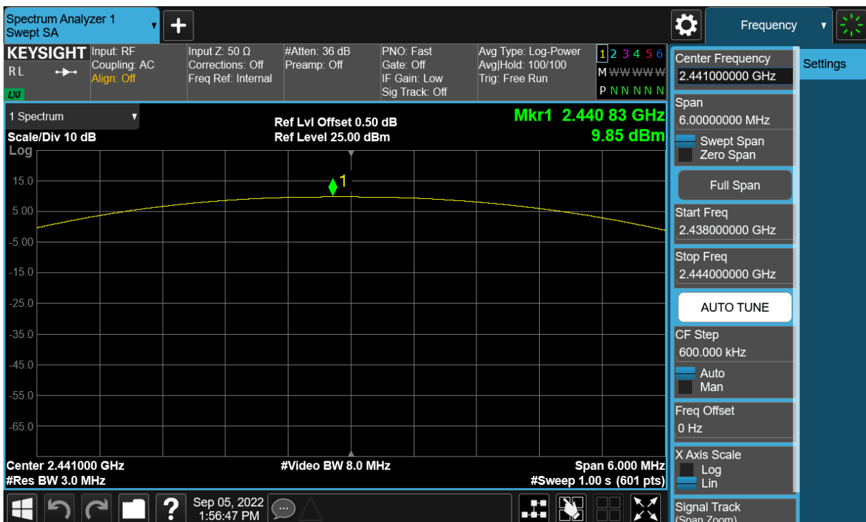
Figure 2: The plots of Maximum Conducted Peak Output Power, 2441MHz, GFSK
