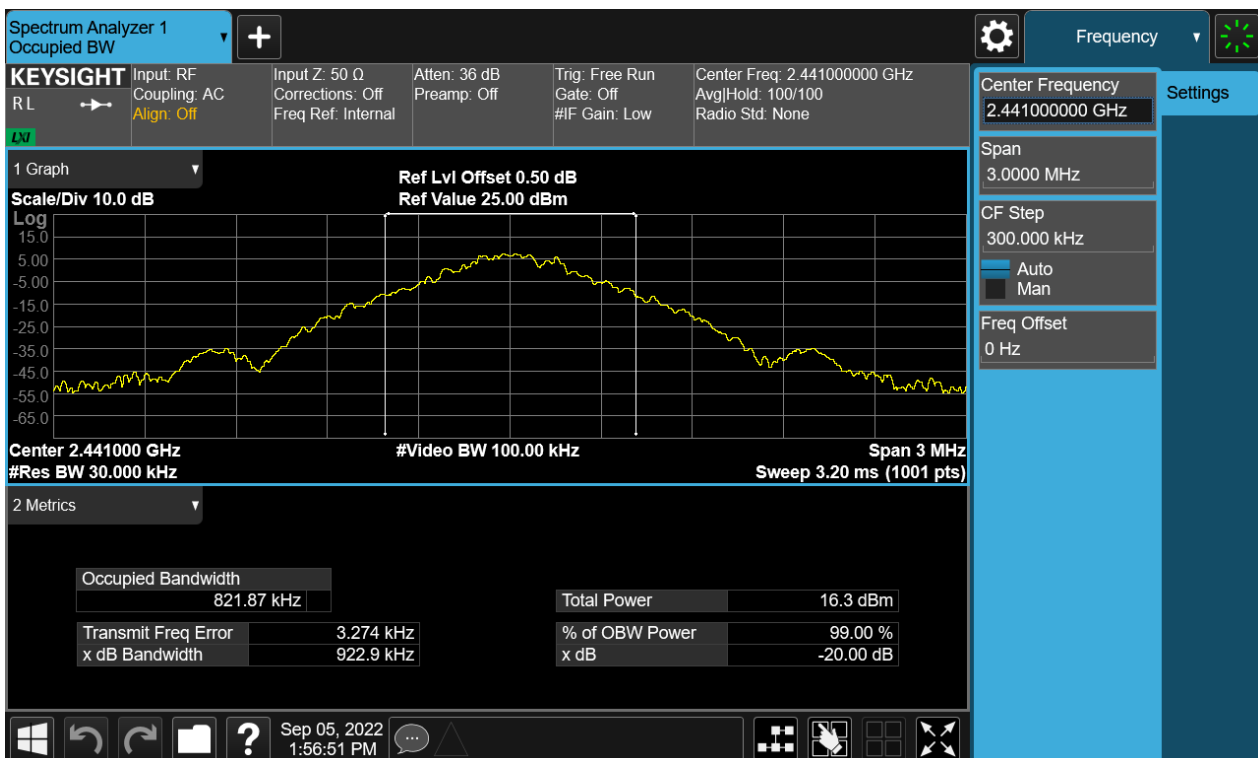
Figure 11: The plots of 20dB Bandwidth and 99% Bandwidth, 2441MHz, GFSK
