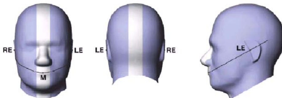
Figure 6.2 Front, back and side view SAM Twin Phantom
