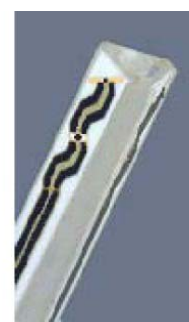
Figure 3.3 Probe Thick-Film Technique
